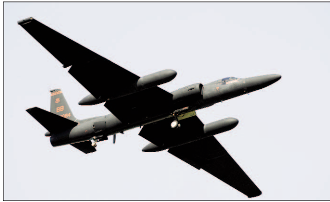
The U-2 is a single-seat, single-engine, high-altitude, reconnaissance aircraft. It is an extremely reliable reconnaissance aircraft, and enjoys a high mission completion rate.
