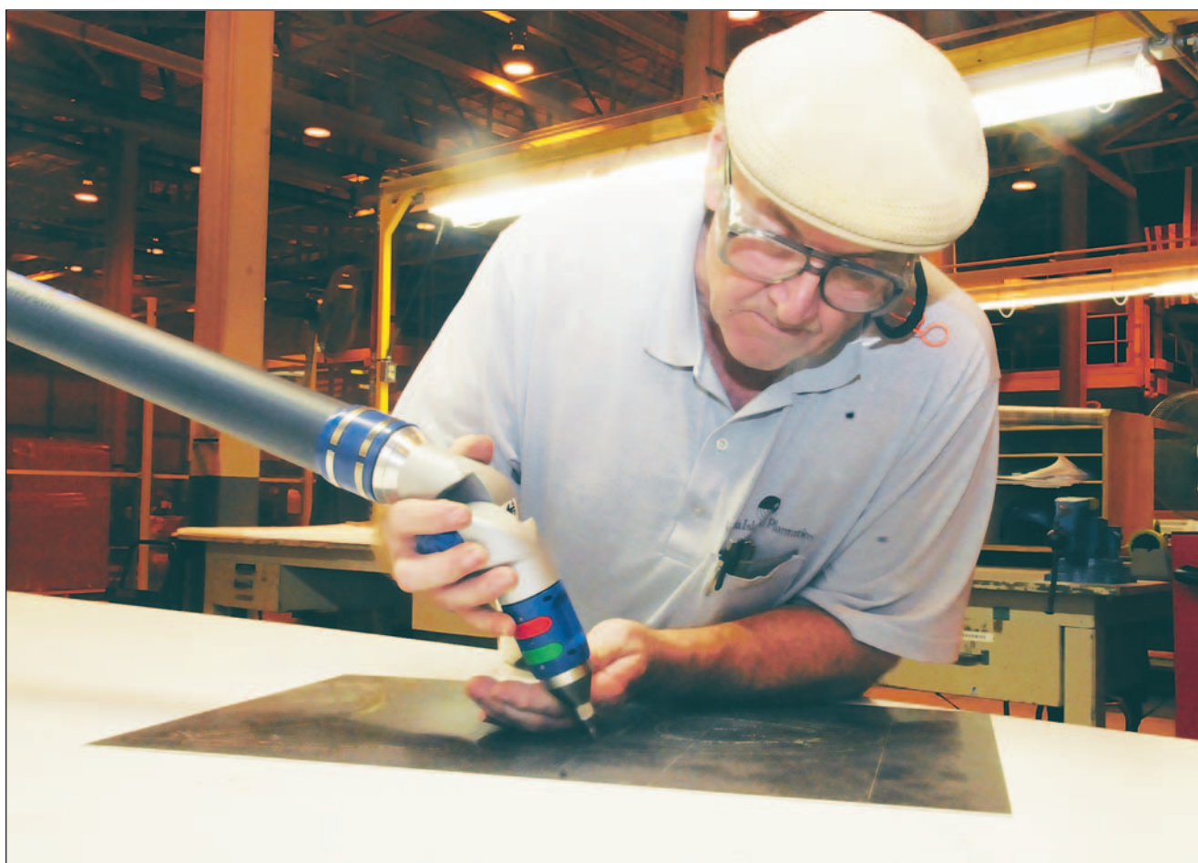
U.S. Air Force photo by SUE SAPP Bernard Stevens uses a computerized measuring machine to get exact measurements to create the geometry so the program can be written for use on the water jet.
