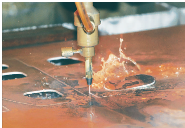
A stream of water cuts a rib for a C-130.
