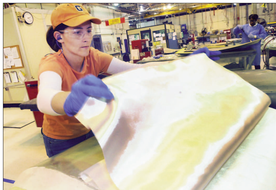
Pamela White puts fiberglass on a composite panel.
