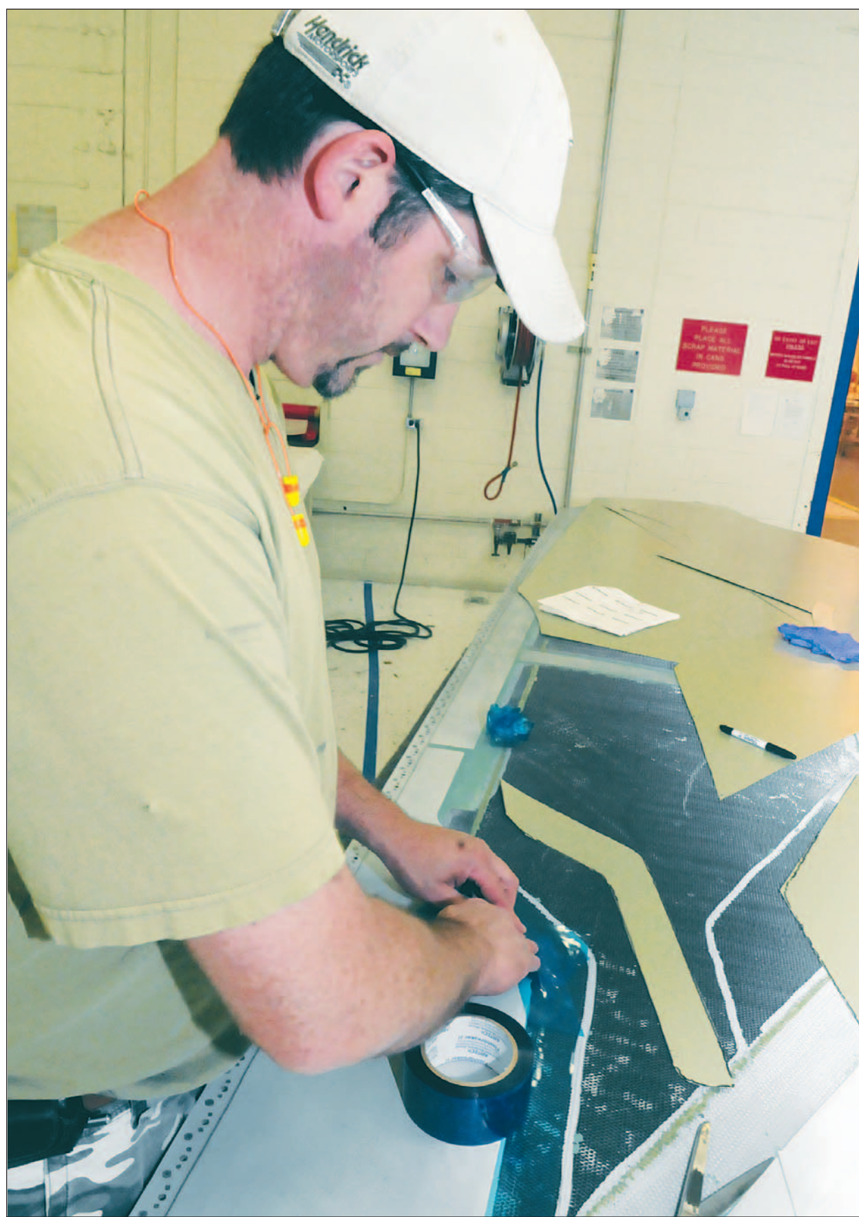
Merrell Ussery makes a template for a C-5 wing tip repair.
