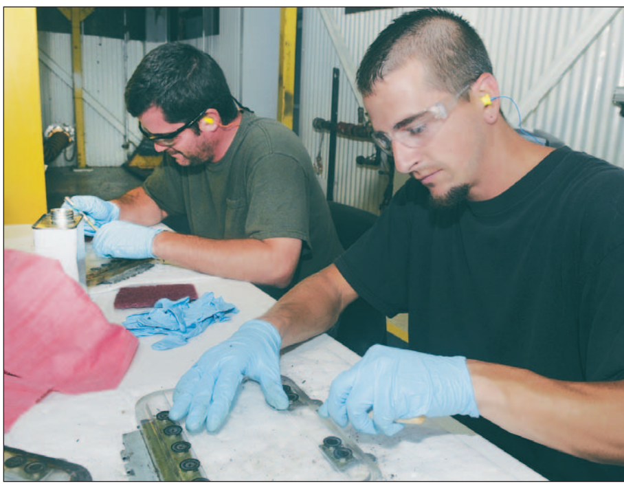
L-R, Casey Medders and Josh Benton clean and put new seals on the C-130's main landing gear inspection window.
