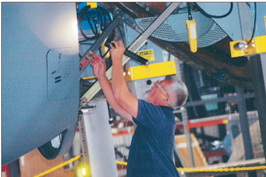
Ken Darsey, inspector, checks for cracks, corrosion and other damage.
