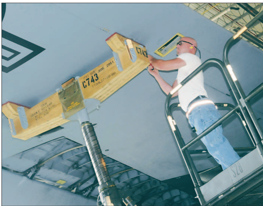
Robert Blizzard works on the hinge pins for the leading edge of the C-130.
