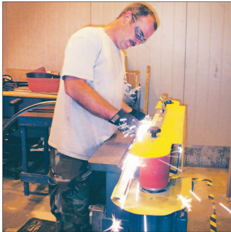
David Stroupe, a sheet metal mechanic, grinds an inconel steel part to required dimensions for the C-130 IRSS.
