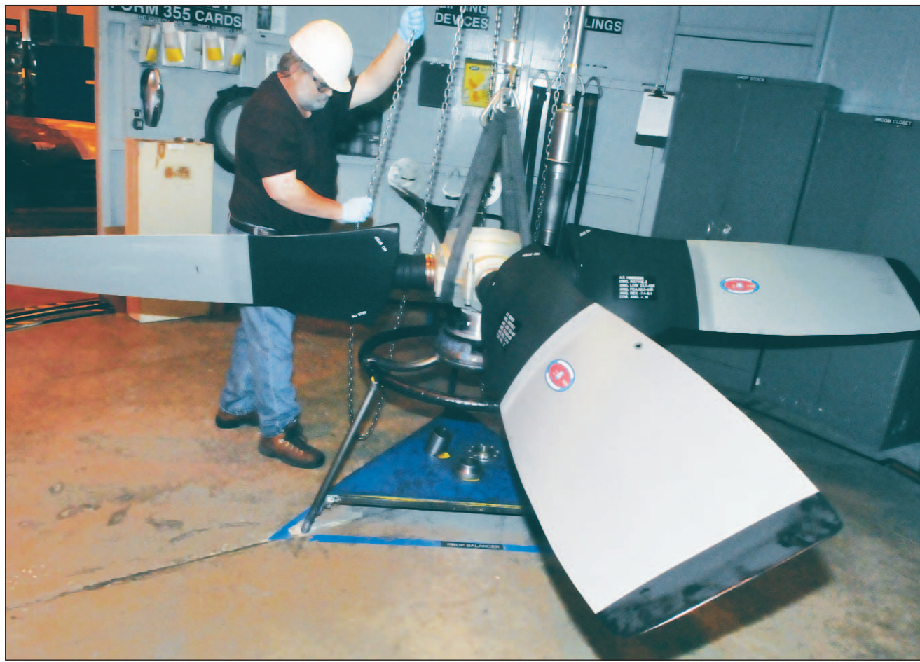
James Kokotilo prepares to static balance a propeller assembly.
