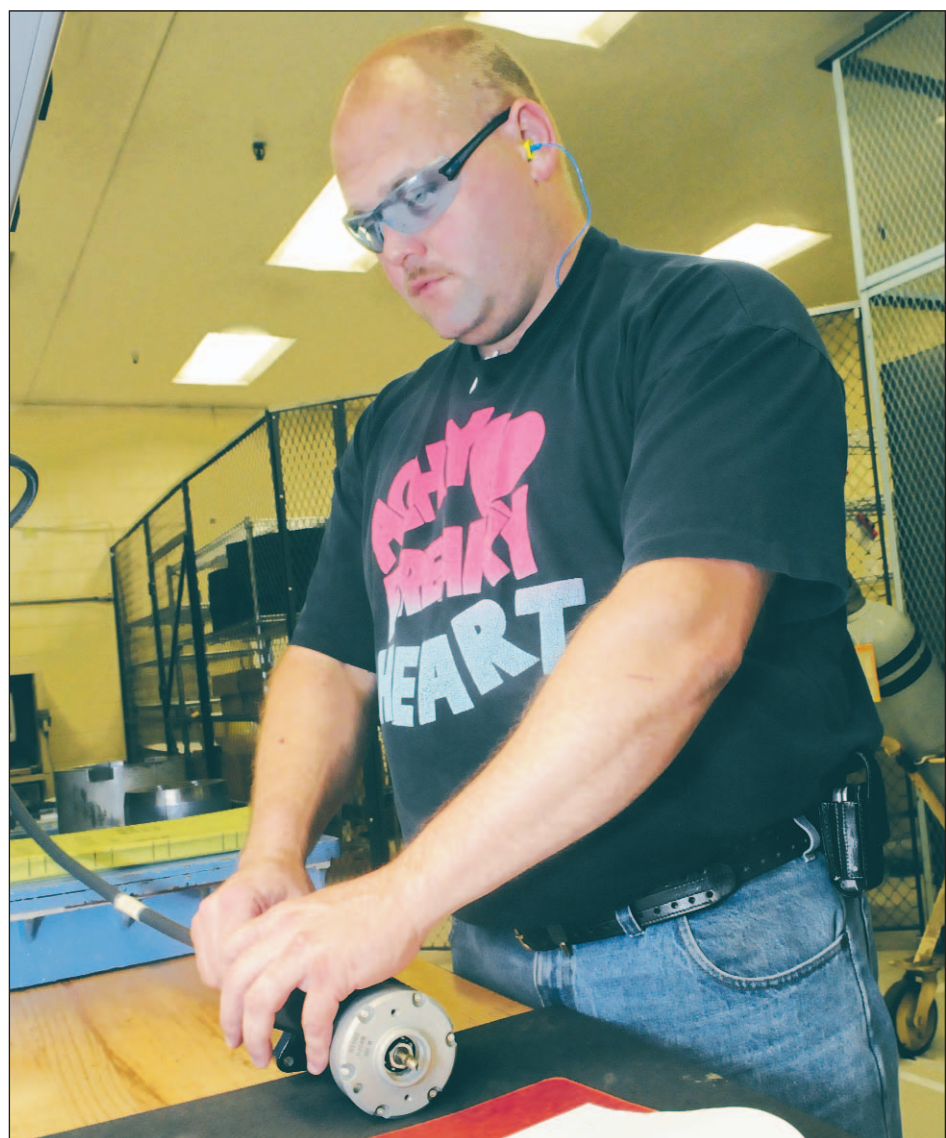
Robert Whaley overhauls an auxiliary control motor.
