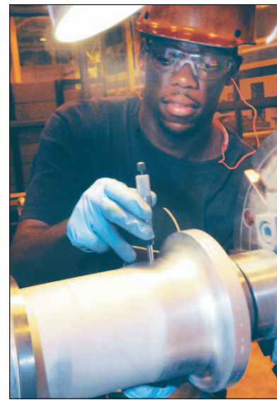
Brian Bradley, measures the outside diameter of a propeller blade so it can be cut down to size.
