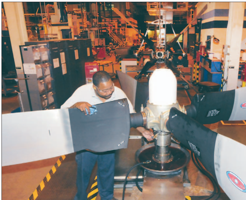
Darrell Carter performs final assembly testing on a C-130 propeller.
