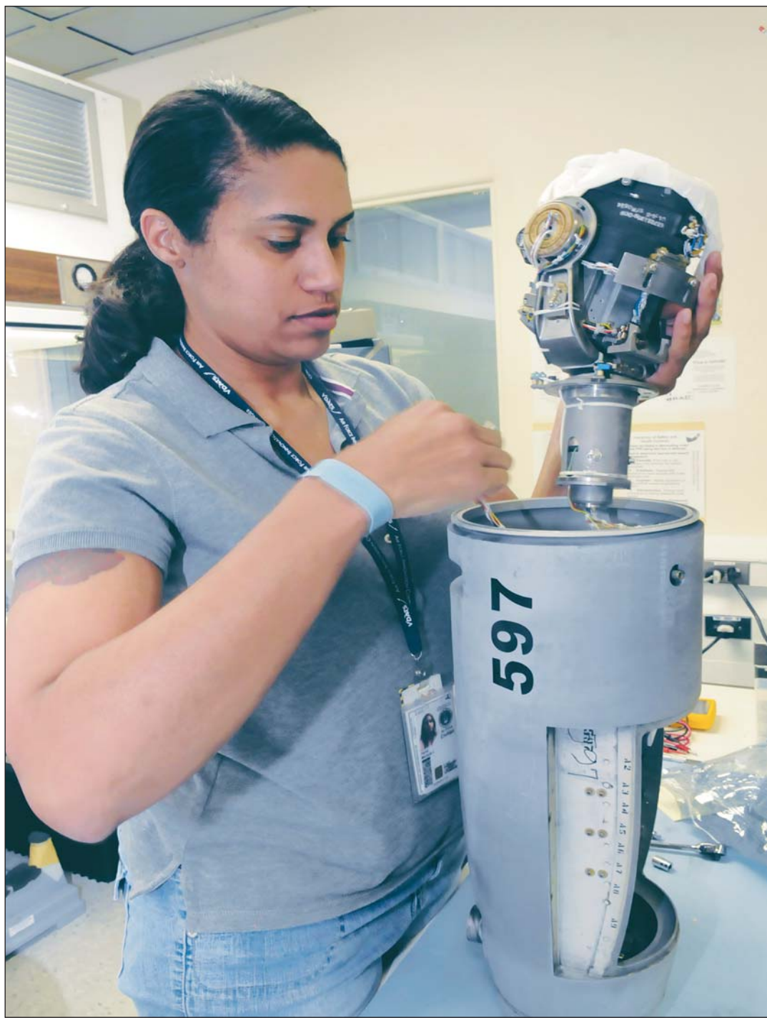
U.S. Air Force photo by SUE SAPP Michele Hand, an electronics mechanic in the 402nd Electronics Maintenance Group, assembles a Pavé Penny pod, which is a targeting pod for the weapons targeting system on the A-10 Thunderbolt II. The pod allows troops on the ground to illuminate targets for A-10 pilots to eliminate. The technology used in the pod is from the 1970s, but remains important to the war effort because of its ability to put troops on the ground in charge of target selection.
