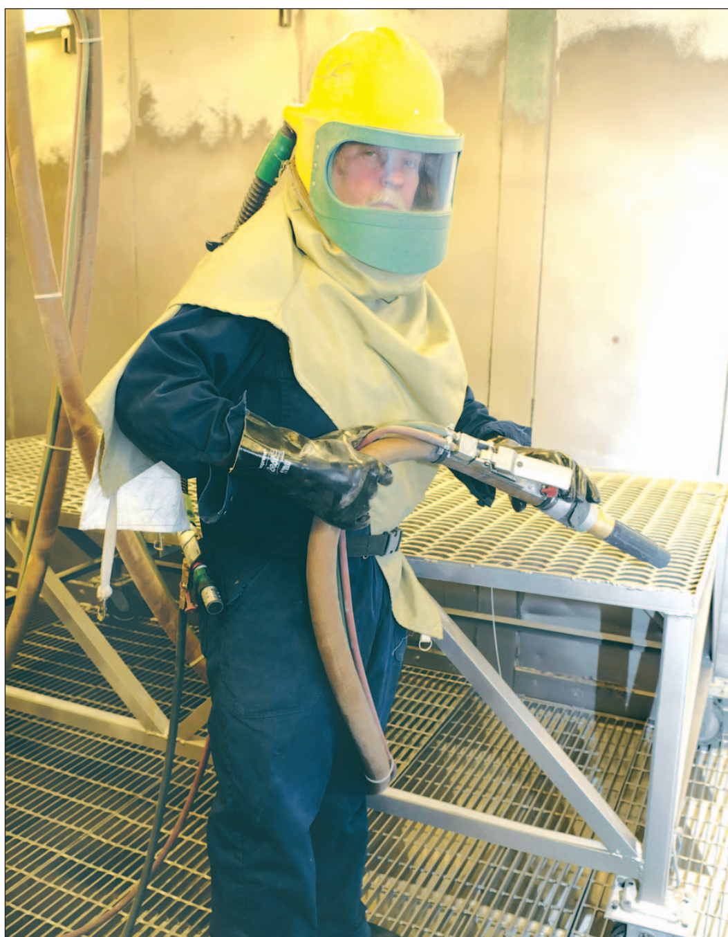
William Brown , electroplater, puts on a special helmet with air supply before going into a blasting booth. If the air supply to the worker is not good, a blue light and loud alarm sounds as a warning.
