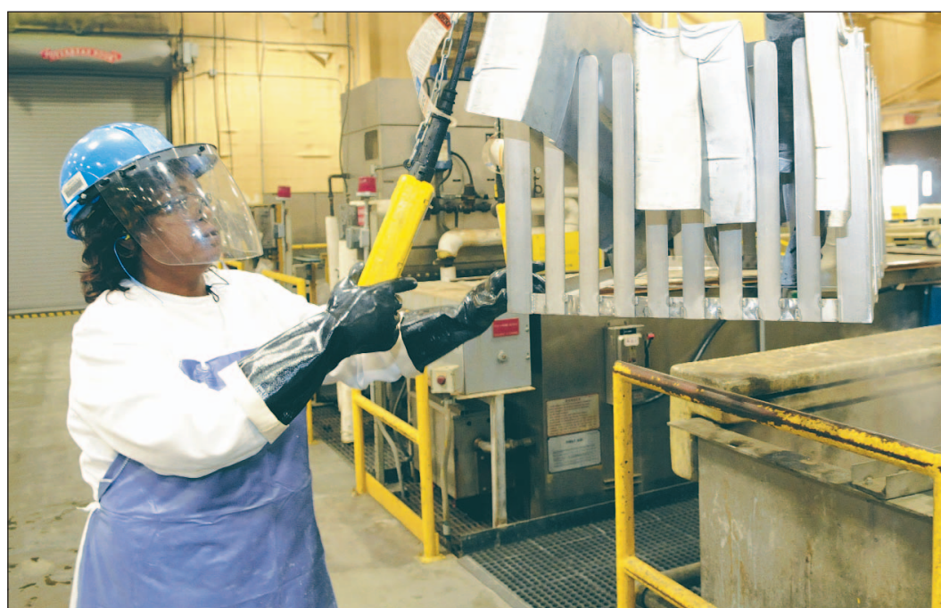
Sarah Lane , electroplater, prepares to dip parts into a degreaser vat for cleaning.
