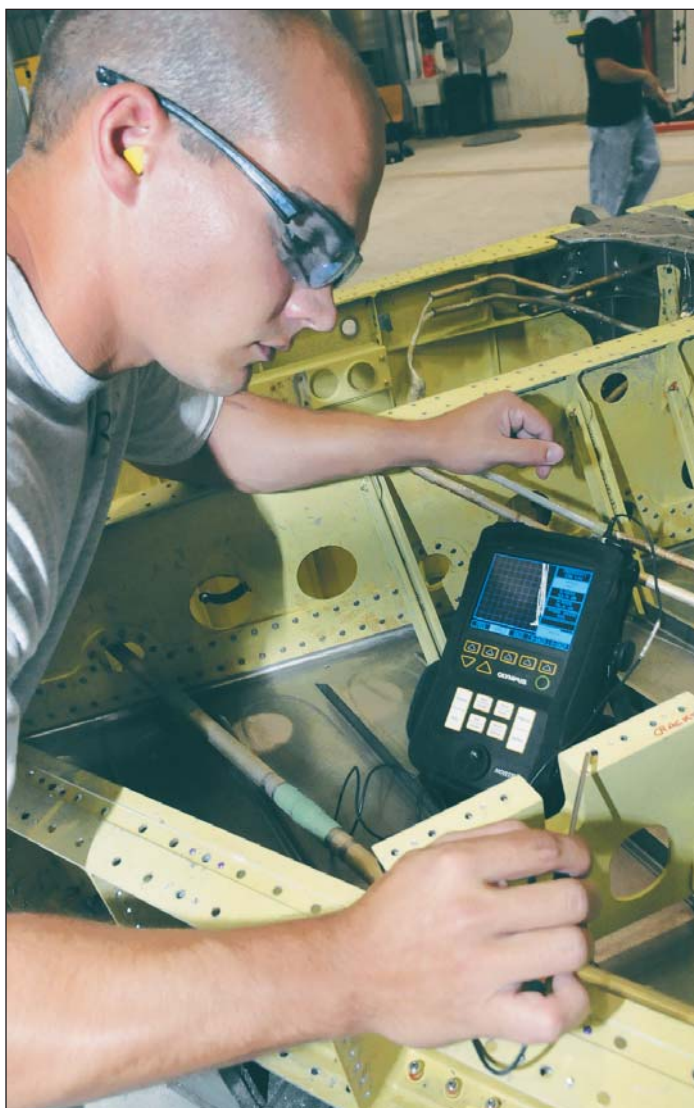
Jason Miller, non-destructive inspector, searches for cracks using an eddy current tester.
