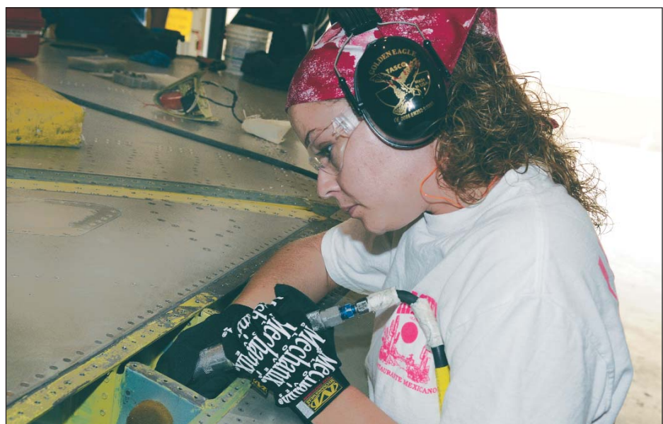
At right, Julie Smallwood, sheet metal mechanic, drills out rivets in the tear down shop.
