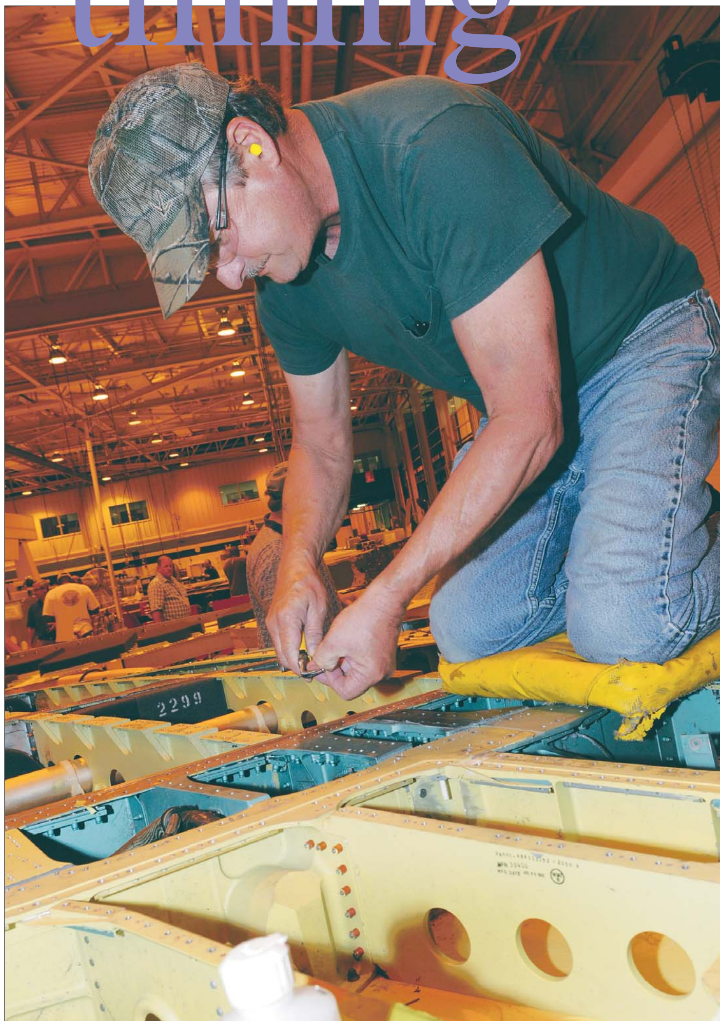
Scott Williams, sheet metal mechanic, installs a bell crank on a flight control in the F-15 Wing Shop.
