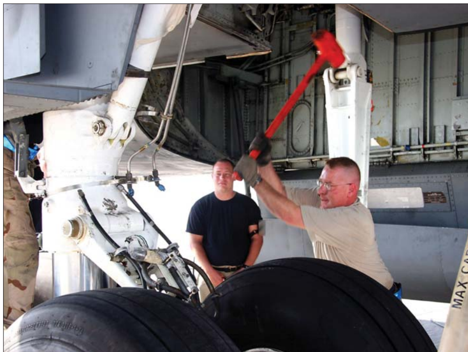
Tech. Sgt. Nathan Darnell (left) observes as Tech. Sgt. James Bernardo carefully lowers the main landing gear strut on a KC-135 Stratotanker to full extension using an 11.5 pound dead blow hammer Dec. 21. The Airmen are assigned to the 380th Expeditionary Aircraft Maintenance Squadron and deployed from the 22nd Aircraft Maintenance Squadron at McConnell Air Force Base, Kansas.
