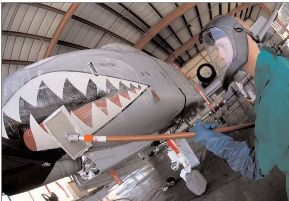
U.S. Air Force photo by AIRMAN ANGELITA LAWRENCE Airmen 1st Class Joshua Norris washes an A-10 Thunderbolt II Nov.19 at the corrosion control wash rack at Moody Air Force Base, Ga. Airmen Norris is a 23rd Aircraft Maintenance Squadron A-10 crew chief.
