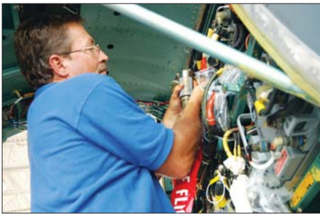
U.S. Air Force photo by SUE SAPP Mark Kitchens attaches the quick adapters to the computers so the cables can be easily hooked up to the tester.
