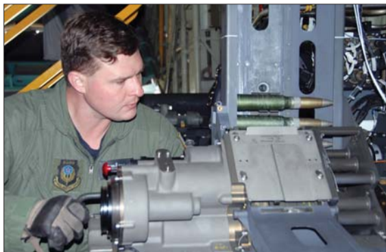
U.S. Air Force photo by CHIEF MASTER SGT. GARY EMERY Technical Sgt. Ben Filek, an aerial gunner with the 19th Special Operations Squadron at Hurlburt Field, Fla., loads a 30 mm Bushmaster cannon aboard an AC-130U Spooky gunship. The 580th Aircraft Sustainment Group's Commando Control Group works to ensure parts like this cannon make it to the aircraft.
