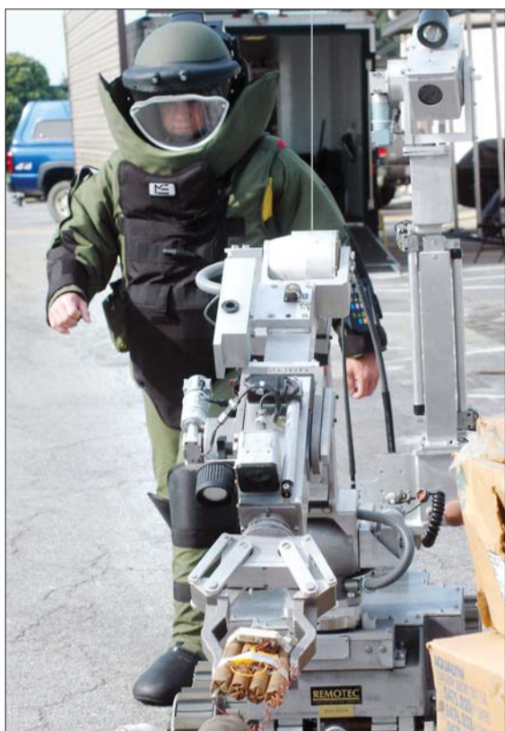
U.S. Air Force photo by SUE SAPP Tech. Sgt. Joseph Fletcher, dressed in an EOD 9 bomb suit, demonstrates the Remotec Andros robot July 13.
