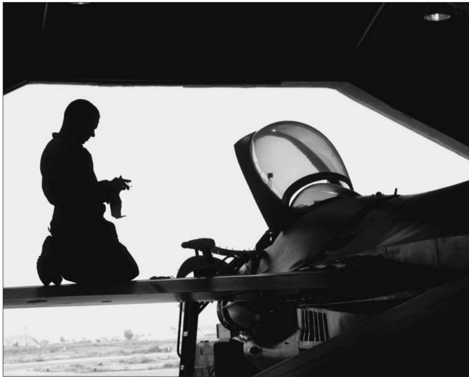
Senior Airman Gil Alicea performs a phase dock inspection on an F-16 Fighting Falcon April 16 at Balad Air Base, Iraq. Maintainers run the inspection every 400 flying hours to keep the aircraft mission-ready. Airman Alicea is with the 332nd Expeditionary Maintenance Squadron.
