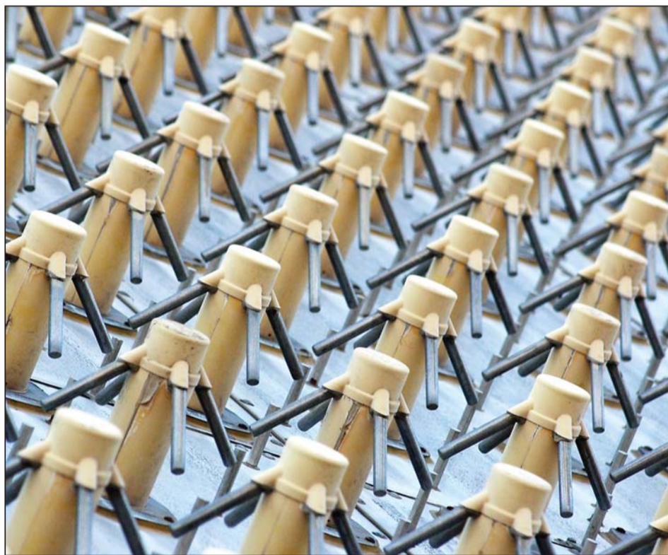
The phased array warning system consisted of the array antennas covering two of the exterior building walls. Each array antenna would send out a pulse.
