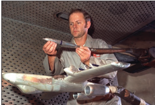
Left, A-10 stores are prepared for testing and evaluation in 4T. Right, one of the first jet engines at AEDC to be studied with the short-duration engine testing technique developed was the TF34. The engine was tested both with the traditional steady-state techniques, in which the engine operating conditions are set at some discrete point before measurements are made, and with the short-duration techniques, in which measurements are made as the engine undergoes controlled changes in operation.
