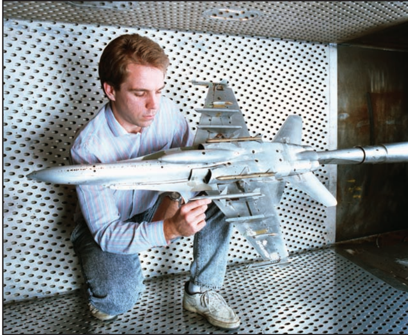
An AEDC engineer checks out a scale model High-speed Anti-Radiation Missile (HARM) attached to a Navy F/A-18 model before the start of a test in 4T. The tests helped ensure that missiles and other stores would safely separate from the aircraft during actual flight.
