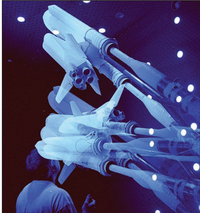
A "blue light" multiple exposure photo of the "full stack" space shuttle in the 16T wind tunnel.
