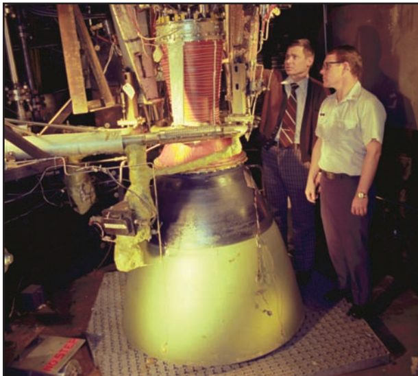
A three-month test program examining the performance of several proposed improvements to the liquid-fueled transtage rocket motor was completed in the same test cell in which the original study was conducted.
