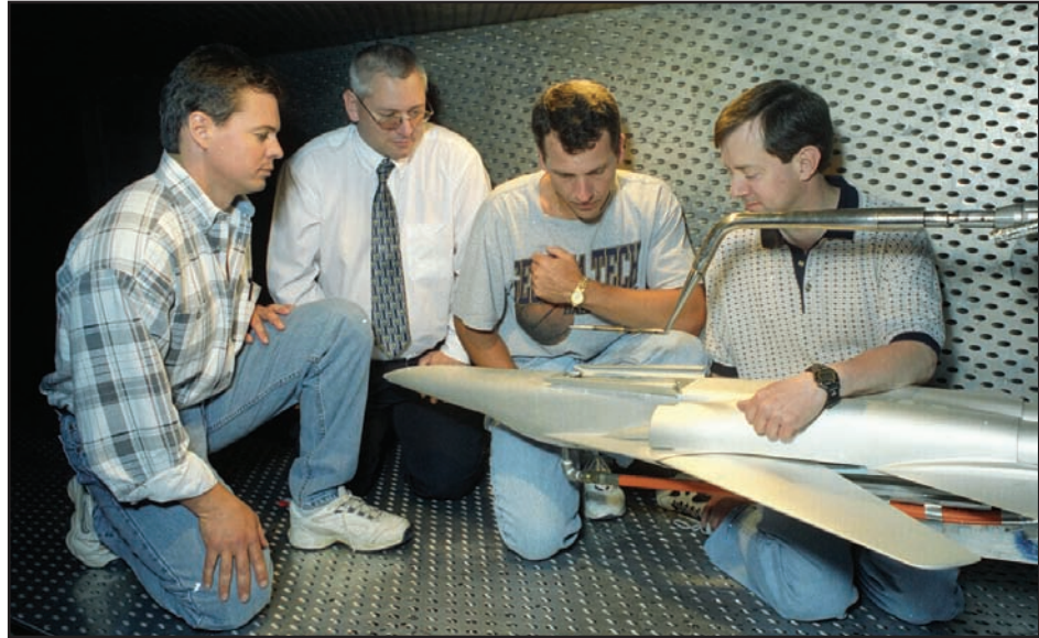
Engineers from the Air Force Research Lab and the Royal Australian Air Force examine an F-111 aircraft and store model in 4T. Since 1960, AEDC has provided design and operational data critical to the F-111 flight-test program development.
