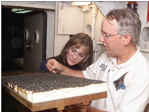
NASA test engineers examine a section of foam paneling of the type used on the space shuttle's main exterior fuel tank during liftoff. Tests on the panels were performed in Tunnel C as a part of NASA's "Return-to-Flight" program. The foam panel was exposed to temperatures above 1,400 degrees Fahrenheit at Mach 4.
