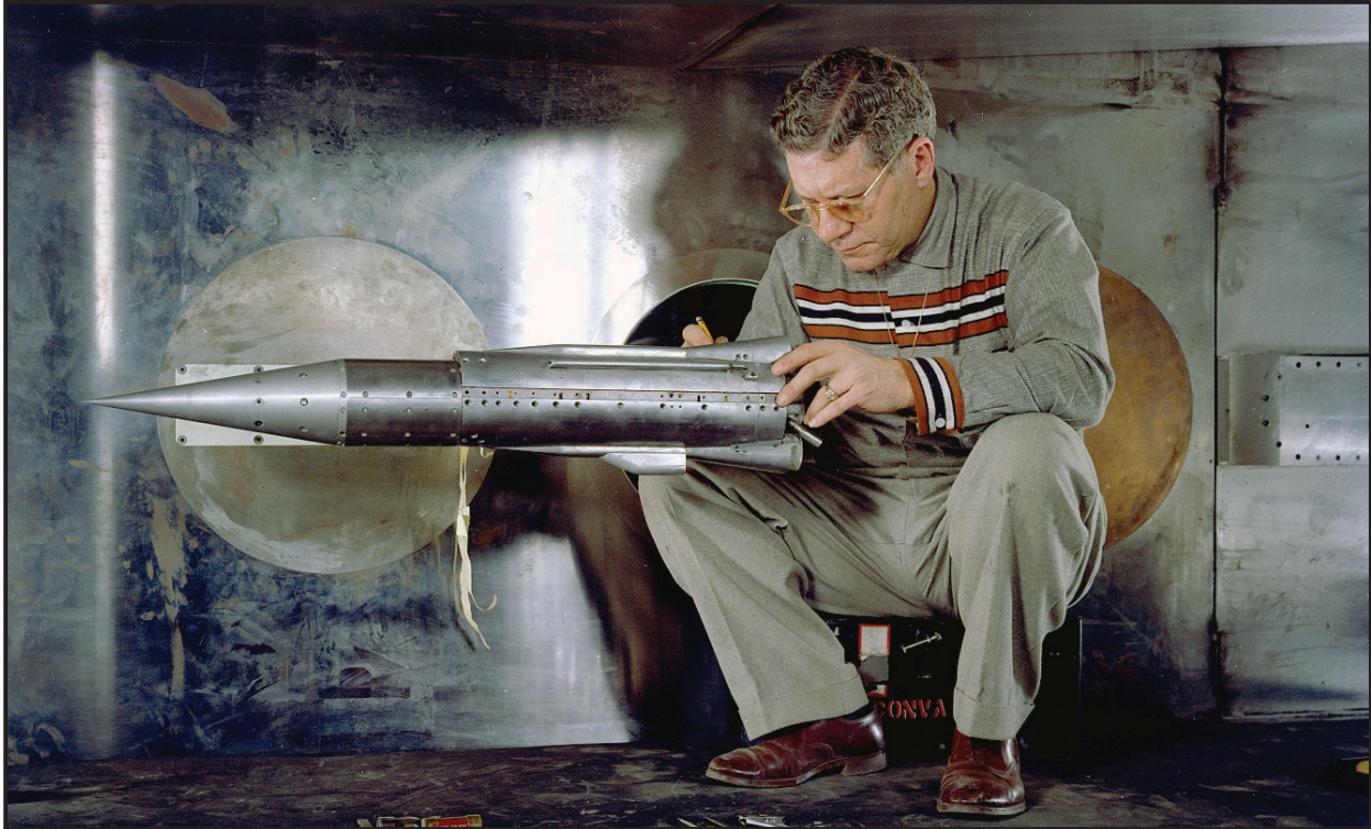
Atlas ICBM base recirculation effects were studied in 1958. The tests were conducted in the center's 40-inch supersonic tunnel using a scale model missile equipped with small rocket engines.
