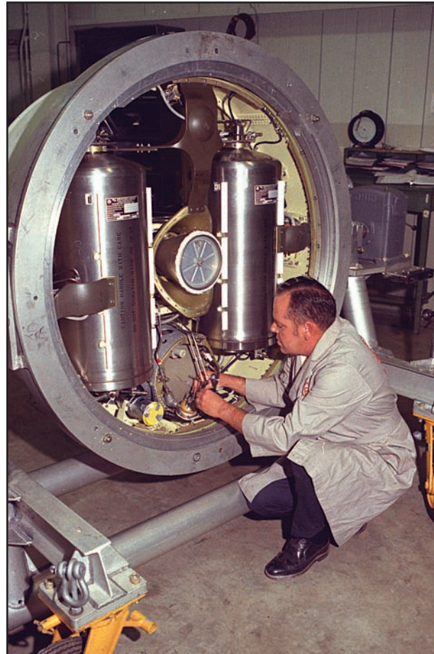
The propulsion system rocket engine PSRE components are checked prior to simulated flight test in J-5 in 1972.
