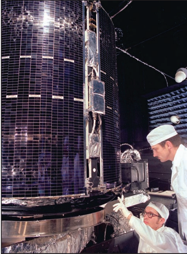
With installation complete and protective plastic wrapping removed, AEDC personnel take a close look at the stowed solar array panels that provide electricity for the NAVSTAR GPS satellite.
