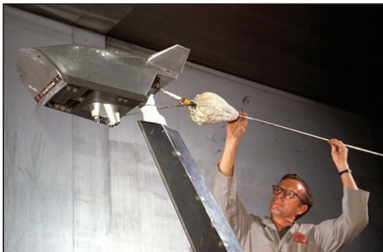
B-1A crew escape capsule is readied for testing.
