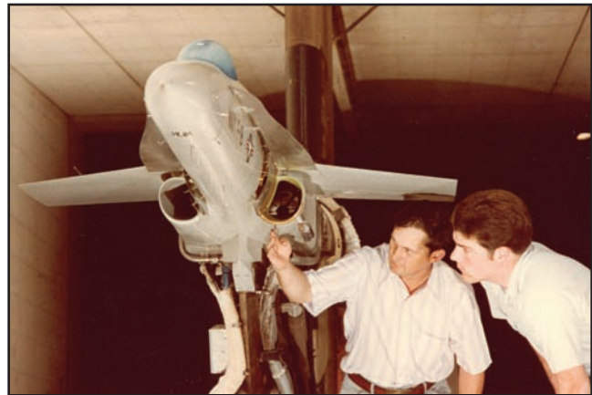
AEDC completed a highly detailed study of the stability and performance of the inlets that provide air to the engines of the F/A-18 fighter. Simulated flight speeds ranged from zero to more than 1,000 miles an hour over a number of angles of attack and sideslip. Nearly 350 sensors were installed in the model to record air pressures. The studies were a continuation of inlet performance tests conducted earlier in both the 16-foot transonic and supersonic wind tunnels in 1977.
