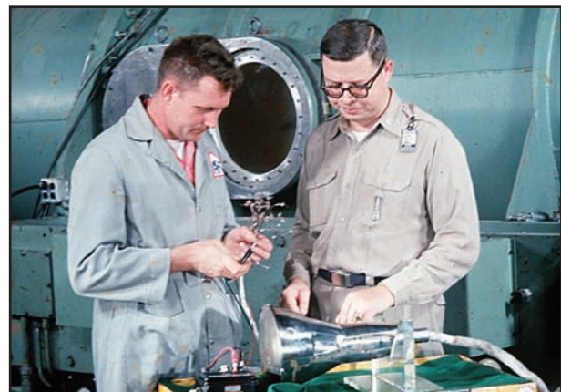
The reentry model of the earth-orbiting, two-man Gemini was tested in many of the center's test units, including the 50-inch Mach 10 wind tunnel.
