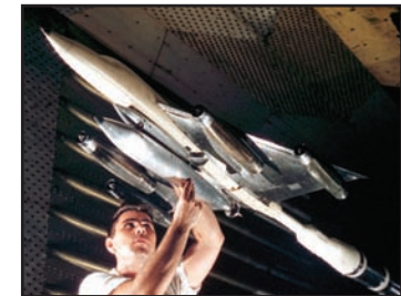
This model of the B-58 Hustler, the Air Force's first operational supersonic bomber, was tested in 16T.
