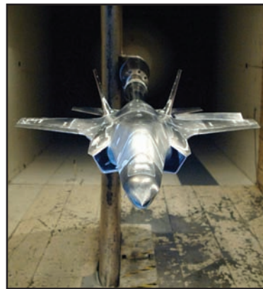
A 12-percent model of the STOVL version of the F-35 Lightning II undergoes aerodynamic load testing in the center's 16T wind tunnel.
