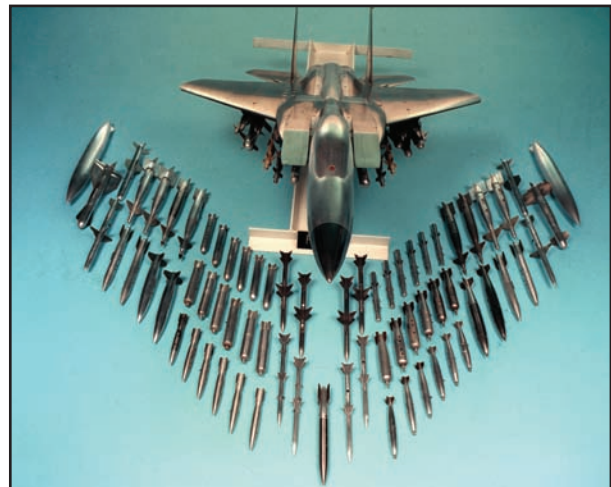
Store separation testing, using 5-percent scale models, began in 1985. More than 500 configurations have been investigated to ensure that the F-15E can safely deliver its wide array of weapons to accomplish its air-to-ground and air-to-air missions.
