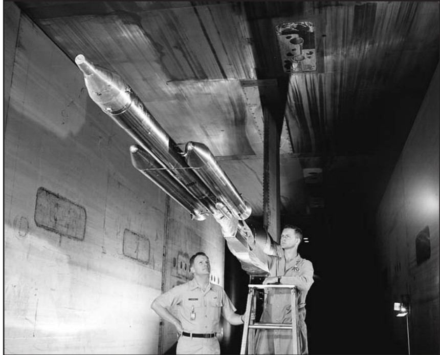
Titan III with a Manned Orbiting Laboratory (MOL) with Gemini is readied for testing in 16S.
