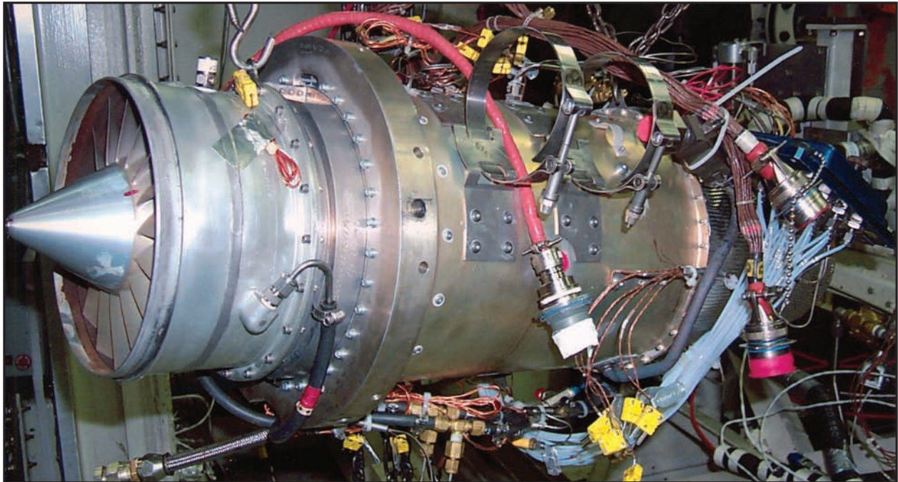
The Williams International F415 engine, installed for testing in test cell T-11, powers the Navy's next generation Tomahawk cruise missile system, the Tactical Tomahawk.
