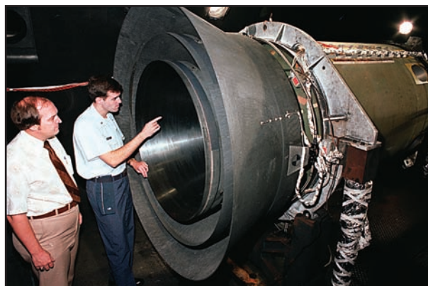
This nested Extendable Exit Cone (EEC) assembly is mated to a Minuteman III solid rocket motor for tests at a simulated altitude of 100,000 feet.
