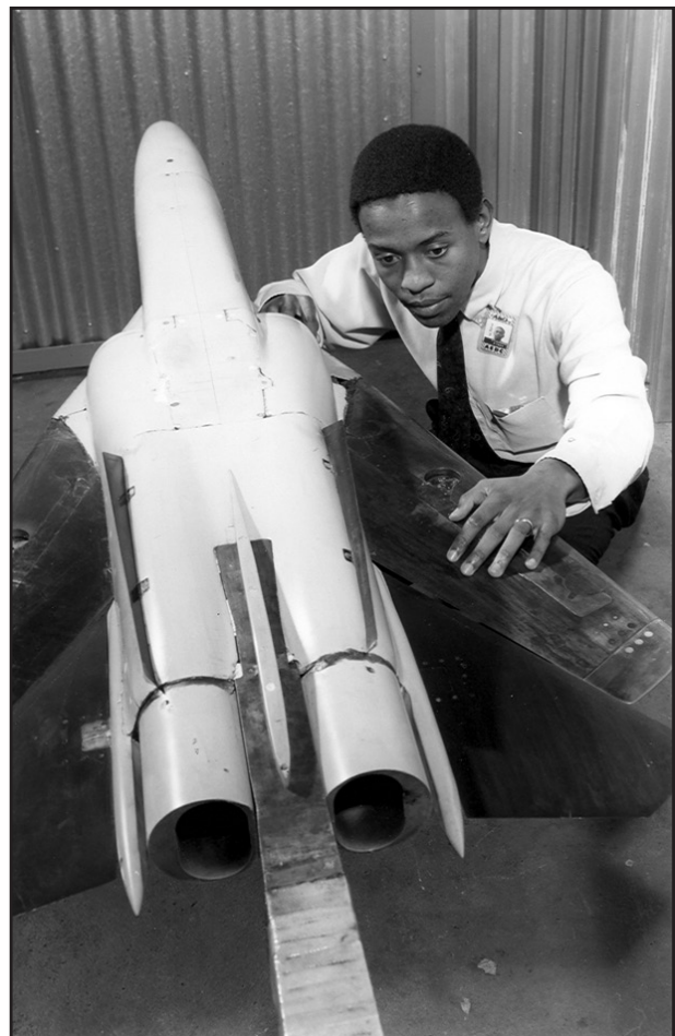
An F-111 swing-wing fighter bomber scale model is checked out by an AEDC project engineer prior to a wind tunnel test in 1969.
