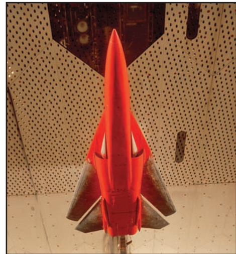
An F-111 wind tunnel model undergoes basic aerodynamic testing and evaluation in 16T in 1968.
