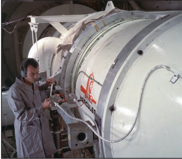
Hercules Poseidon second stage model undergoes testing in the J-5 test cell in 1968.
