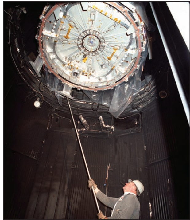
An AEDC rigger helps lower an ISS component – a common berthing mechanism – into the 12V chamber in 1995.
