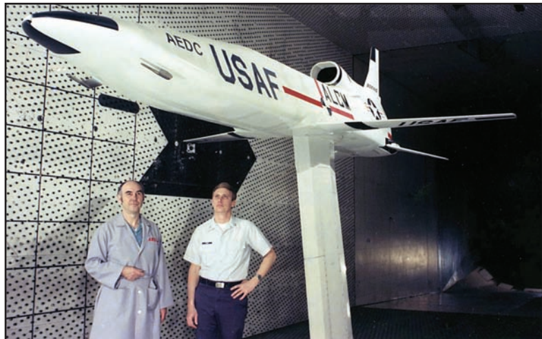
As a preliminary to its successful first flight on March 5, 1976, a full-scale model of the ALCM was tested to verify the missile's operation under simulated launch conditions. Of principal interest in support of the flight program were the ability of the missile's aft control surfaces to deploy and its jet engines to start in midair. Additional tests were also conducted to examine control surface deployment, engine-inlet compatibility and low-temperature engine starting characteristics over a wide range of launch conditions and flight attitudes. The tests were conducted in 16T.
