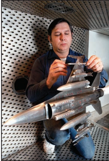
Left, last-minute adjustments prior to a wind tunnel test in 4T on an F-16 aircraft model configured with various store models. Right, the GE F110-GE-129 engine is shown in the J-2 engine test cell. The engine used improved materials and controls to increase performance up to 20 percent over the F110-GE-100 engine used in the F-16 Fighting Falcon. The tests simulated the full range of the engine's flight envelope up to Mach 2.5 and 65,000 feet altitude.
