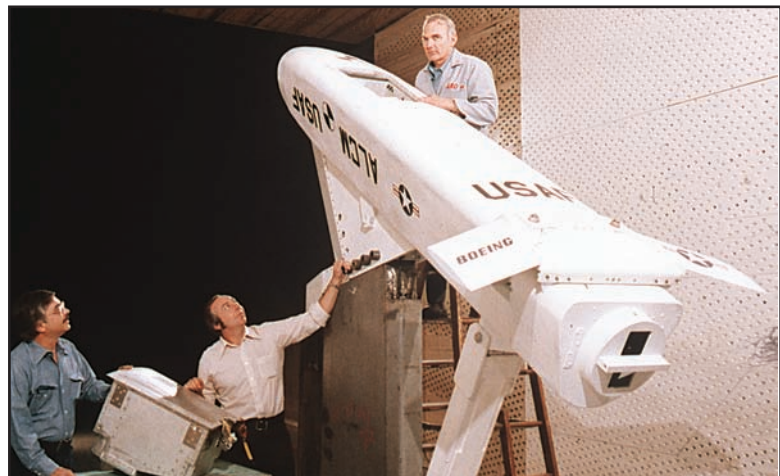
An ALCM was tested in 16T prior to its first flight. The full-scale weapon is shown installed in 16T in 1976.
