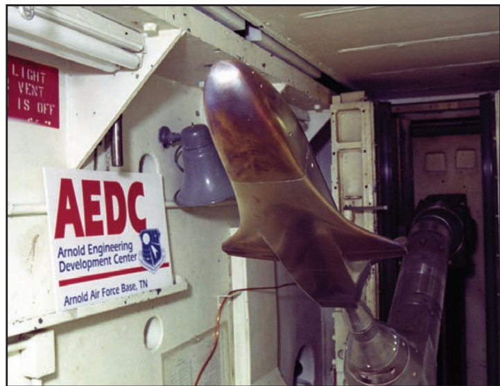
A wind tunnel test in VKF used a 6-percent scale model of Boeing's X-37 to investigate the aerodynamic forces and moments of the vehicle and aerodynamic jet interaction effects from plumes of small reaction control system jets on the model.
