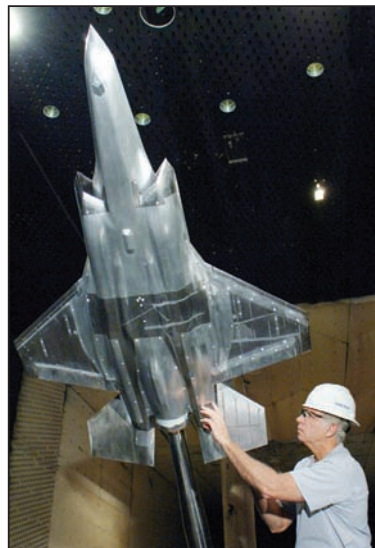
A Lockheed Martin engineer inspects the JSF model during a break in aerodynamics load testing in wind tunnel 16T.
