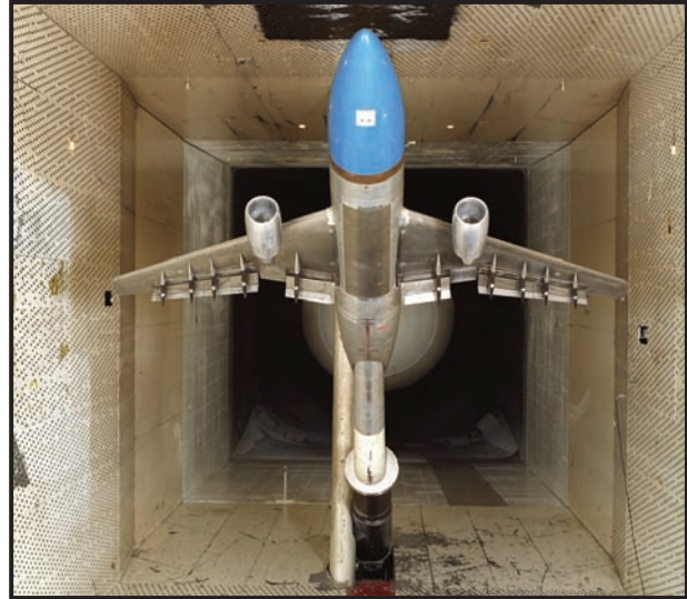
A British A300-B2 Airbus model undergoes wind tunnel testing and evaluation in 1996.
