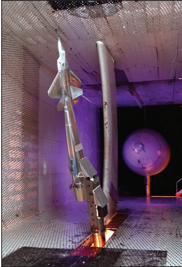
An F-22A aircraft model is maneuvered to a very high angle of attack during wind tunnel testing in 16T. This test helped to define performance and aircraft stability and control.
