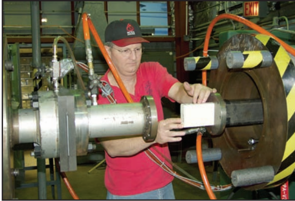
A foam projectile is loaded into the 86-foot-long rectangular barrel of the center's Bird Impact Range in preparation for tests for the space shuttle "Return-to-Flight" program.
