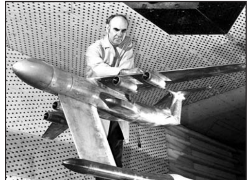
A test technician checks out a seven-foot-span scale model in 16T in 1978. The tests were made to check the feasibility of improving aerodynamic performance of a stretched version with 23-foot longer fuselage.
