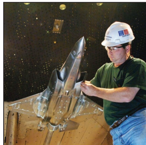
An ATA craftsman examines the STOVL F-35 model in wind tunnel 16T during a model change. The information from this testing, the final entry in a series of tests, went into a large database to refine and validate the aircraft designs for flight testing.
