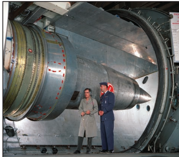
The GE TF39 engine for Air Force's C-5A transport is readied for qualification test in the J-1 engine test cell.
