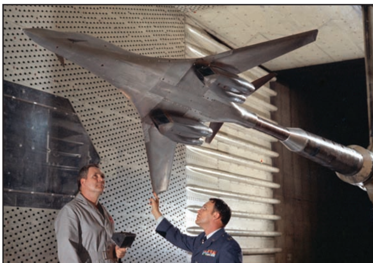
AEDC engineers inspect the model as it is pitched to various angles of attack and roll prior to a test run. In 1972, the series of tests supporting development of the Air Force's B-1 advanced bomber involved this 6-percent scale model in 16S and 16T. The effects of model size were investigated by comparing data from the tests of the two differently scaled models as a basis for more accurate predictions of flight performance.
