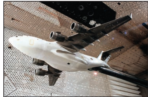
A highly instrumented C-17 model, with 15 remote-controlled surfaces was tested in 16T in 1983.
