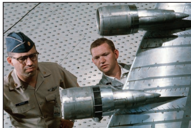
This was one of the C-5A test programs conducted in PWT that were cited by then General James Ferguson, commander, Air Force Systems Command, in support of his views on the continued development of aerospace testing facilities. The test model was a "semi-span" model at 1/18th scale. Included were the left wing with its two engines and half the fuselage. This model was wired up with over a thousand pressure sensors distributed around the surface and leading to remote recording devices.
