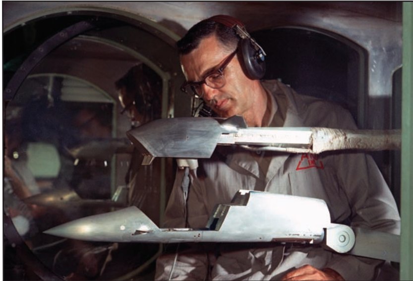
The B-1A crew escape capsule is mounted on a remote-controlled support capable of movement in three directions. The model was subjected to airflow at 1.5 and 2.25 times the speed of sound as the flow field around the capsule and simulated aircraft were studied.
