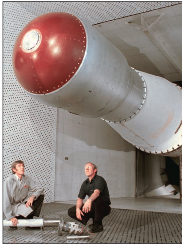
Wind tunnel tests to examine deployment of a mechanical device that changes the aerodynamic shape of the Trident missile was completed in 1975. The AEDC tests were conducted by mounting a full-scale nosecap on the scavenging scoop of 16T. Normally the scoop is used to remove combustion products from the closed-loop tunnel during jet or rocket engine tests. It was adapted into a support structure because of the size and weight of the nosecap. On the floor of the tunnel are an extended aerospike assembly and one in the retracted position as it is fitted into the nosecap during the underwater phase of its flight.
