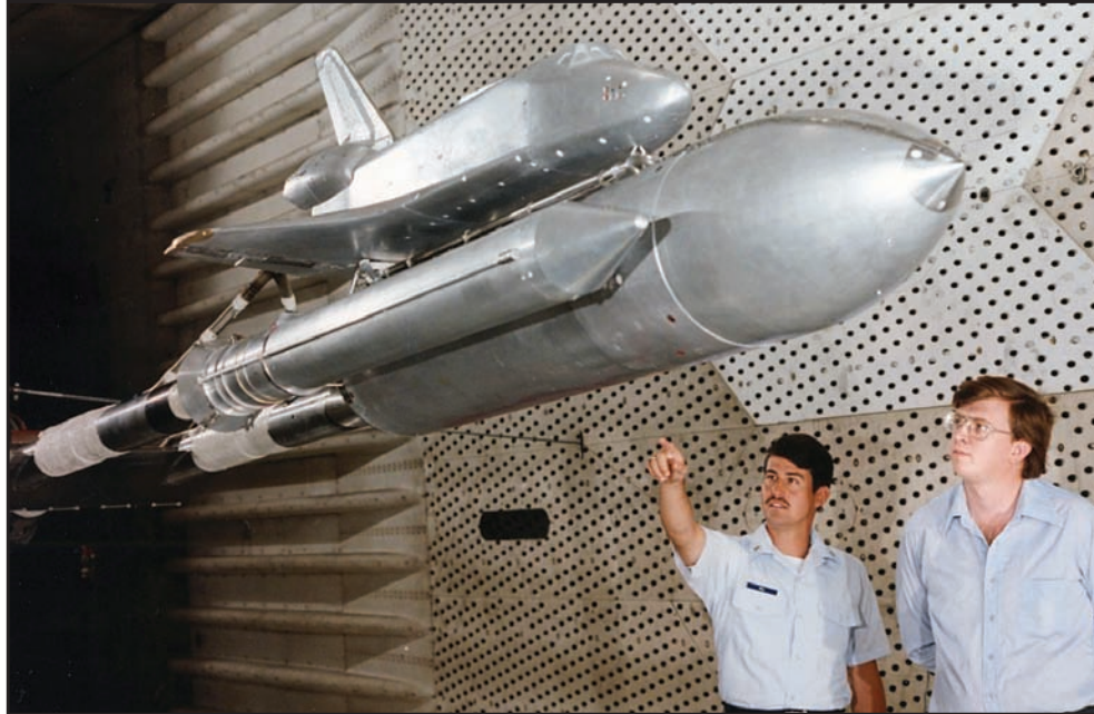
A 0.0175-percent scale model of NASA’s space shuttle orbiter, solid rocket booster and external fuel tanks underwent aerodynamic testing in tunnel 16T.
