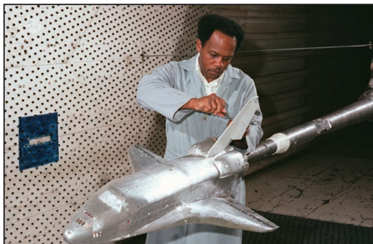
A NASA space shuttle orbiter model was tested in 1978 in tunnel 16T. This series of tests provided data on the effects of vertical stabilizer deformation on flight control.
