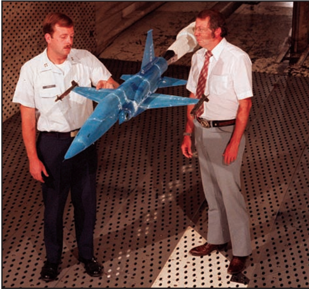
A 10-percent scale model of Northrop's F-5G fighter was tested in 16T to define the aircraft's aerodynamic performance over a wide range of simulated altitudes.
