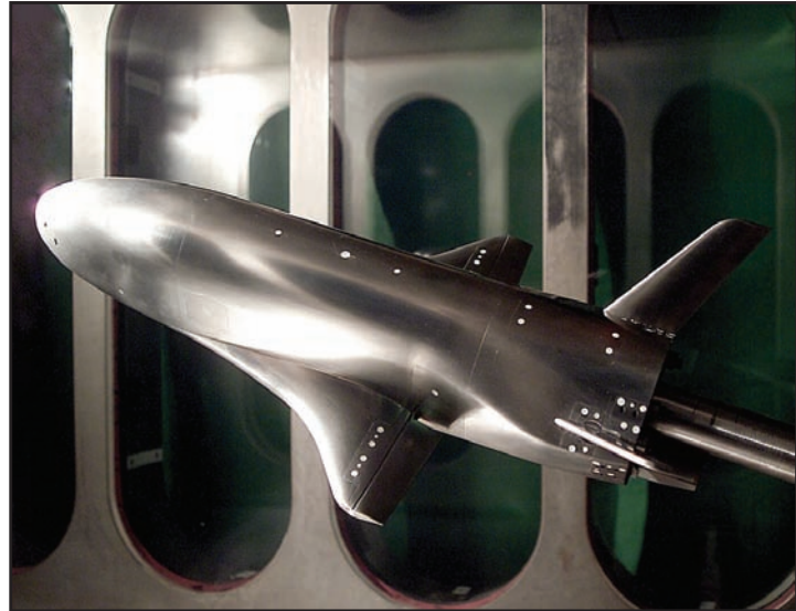
A 6-percent scale model of NASA's X-37 underwent testing in tunnels A, B and C to establish how redesigns to the demonstrator spacecraft's control jet nozzles and body flap effected its aerodynamics during reentry into and through the Earth's atmosphere.
