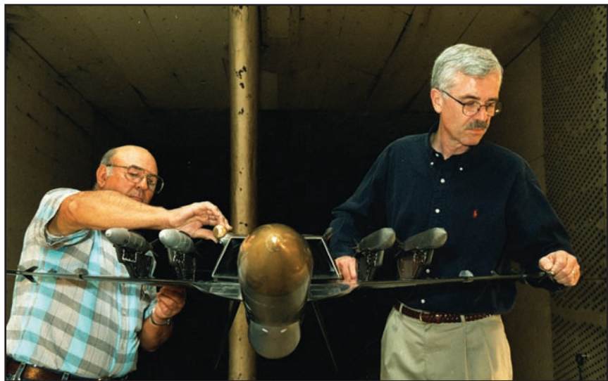
AEDC personnel prepare an F/A-18E/F model aircraft in 16T for a carriage loads test.
