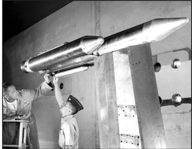
A scale model of the Titan III booster system for the X-20 Dyna-Soar manned orbital glider is mounted for testing in the Propulsion Wind Tunnel's 16-foot supersonic wind tunnel (16S) in 1963.
