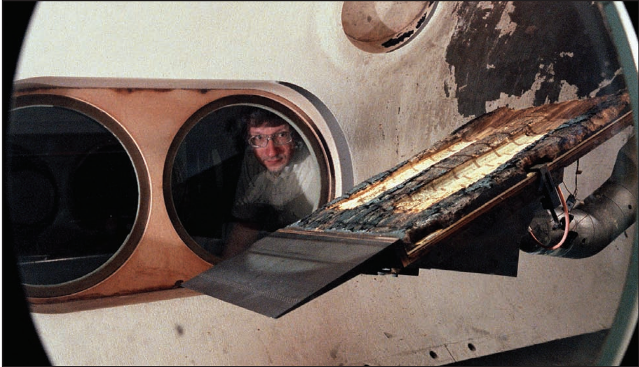
Foam insulation for the external fuel tank of NASA's space shuttle underwent material testing in VKF's hypersonic Tunnel C.
