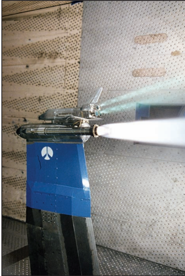
A 2.25-percent scale model of NASA's space shuttle launch vehicle is shown during hot rocket plume simulation tests in 16T. Aerodynamic effects generated by selected orbiter main engine-out configurations were determined. Exhaust from the orbiter main engines was simulated by short-duration burn of gaseous hydrogen and oxygen. Solid rocket booster (SRB) plumes were generated by burning a mixture of gases designed to match thermal and propulsive properties of the actual SRB plumes.
