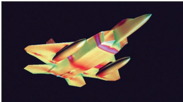
AEDC engineers used CFD to determine the flow fields around the F-22A. Here a fighter is shown carrying external fuel tanks.
