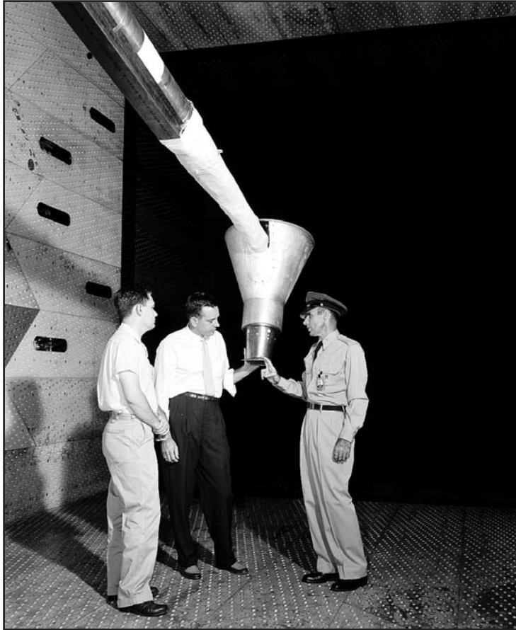
The Project Mercury model was tested in the center's 16T wind tunnel.
