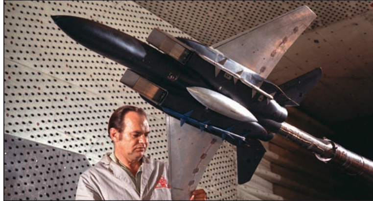
Seven F-15 design changes were verified in tests in 16T. AEDC did extensive support during the research and development stage of the F-15 program.
