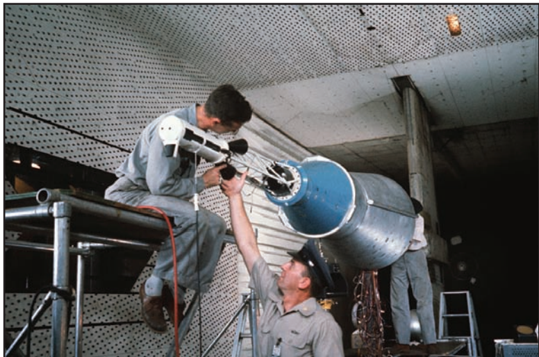
A 1960 Mercury escape tower test in 16T improved stability to prevent tumbling in the event of an emergency abort during satellite launch.
