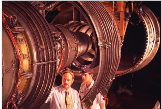
Left, A-10 stores are prepared for testing and evaluation in 4T. Right, one of the first jet engines at AEDC to be studied with the short-duration engine testing technique developed was the TF34. The engine was tested both with the traditional steady-state techniques, in which the engine operating conditions are set at some discrete point before measurements are made, and with the short-duration techniques, in which measurements are made as the engine undergoes controlled changes in operation.
