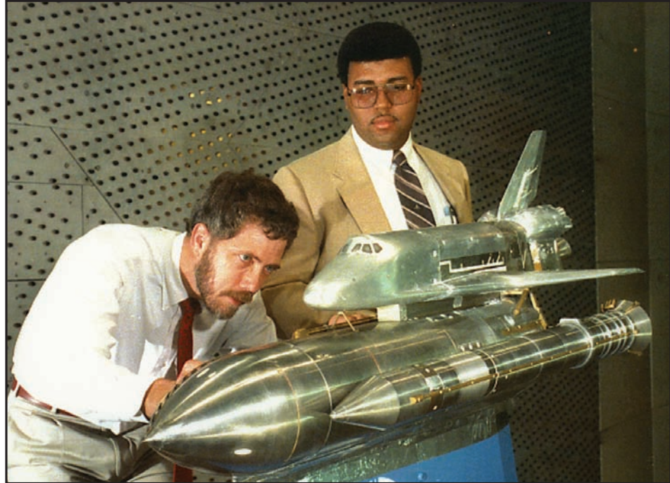
Test personnel check out a model of the space shuttle with fuel tank and solid rocket motors in 16T prior to a test in 1988.
