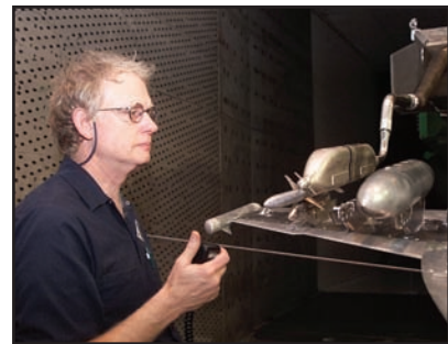
An outside machinist speaks through a microphone to test personnel in the 16T control room who are operating the metal arm, or sting, with a wing store above the EA-18G model.
