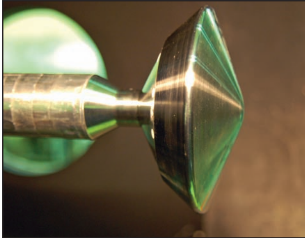
Above, a 1/30 scale model of the aeroshell configuration for the Mars Science Laboratory at AEDC's Hypervelocity Wind Tunnel 9 Facility. Right, a Schlieren image shows the density gradients in the laminar/turbulent boundary layer of the aeroshell configuration.
