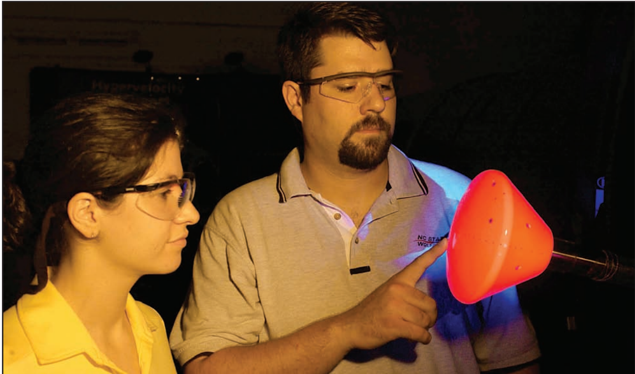
A University of Maryland graduate student and an ATA engineer examine the illuminated TSP coating on the NASA CEV model prior to a run at Tunnel 9.
