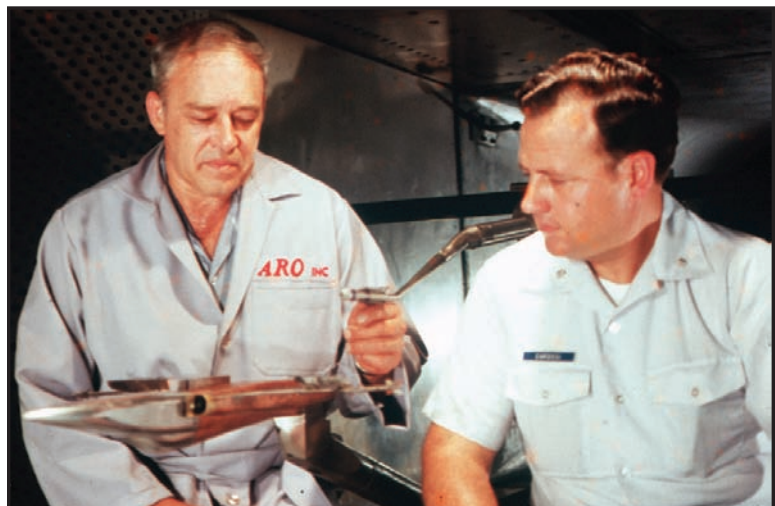
The F-5 underwent store separation testing in AEDC's 4-foot transonic wind tunnel in the early 1970s.
