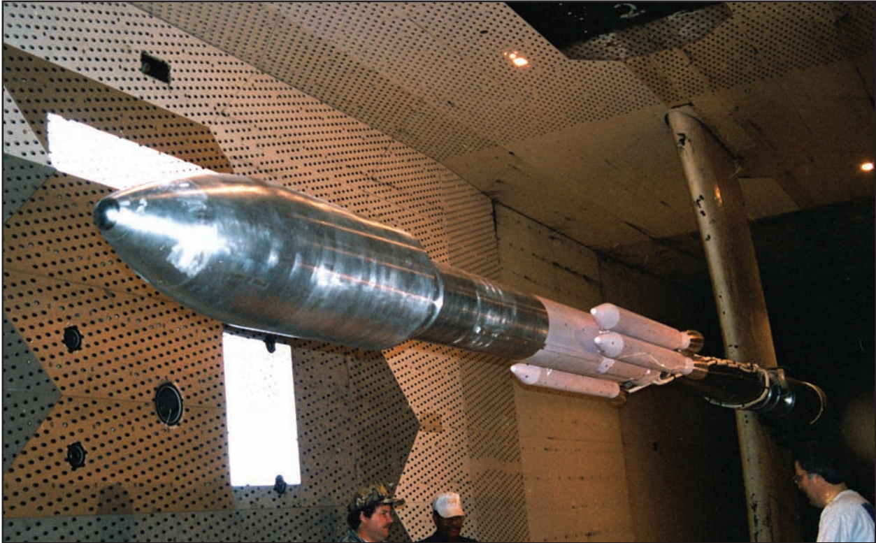
Lockheed Martin Astronautic designers and AEDC engineers conducted aerodynamic tests on the Atlas V in wind tunnel 16T to help Lockheed Martin determine detailed local acoustic and vibration environments as well as whole vehicle buffet load environments.
