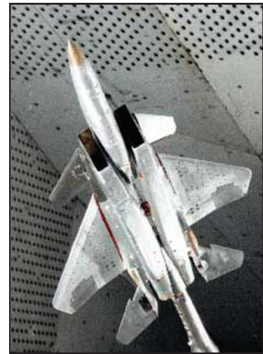
F-15 Eagle Short Take-Off/Landing demonstrator models were tested at AEDC for several years prior to the first flight in 1989. This 1985 photograph shows a model in 16T.
