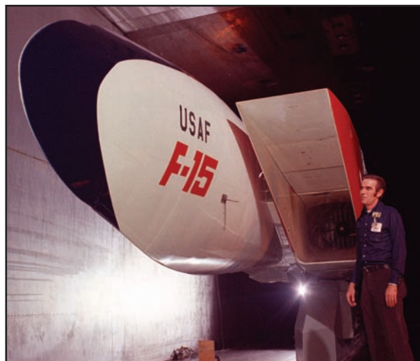
A full-scale F-15E inlet and operating engine were tested in 1972 in 16S. The tests demonstrated the compatibility of the F100 engine with the F-15’s variable geometry inlet.
