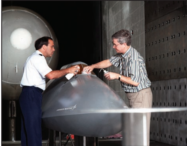
AEDC engineers clean the window containing the sensor for an Advanced Infrared Search and Track system on an F-22A aircraft model. The aero-optical performance of the system was validated during wind tunnel testing at AEDC.
