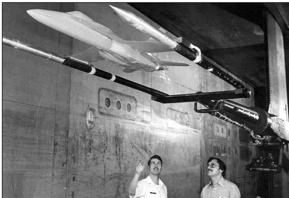
Wind tunnel tests in 16S using the F/A-18 as a test vehicle investigated possible improvements in performance of jet fighters – improvements which may be gained by equipping an aircraft with rectangular jet nozzles instead of round ones.
