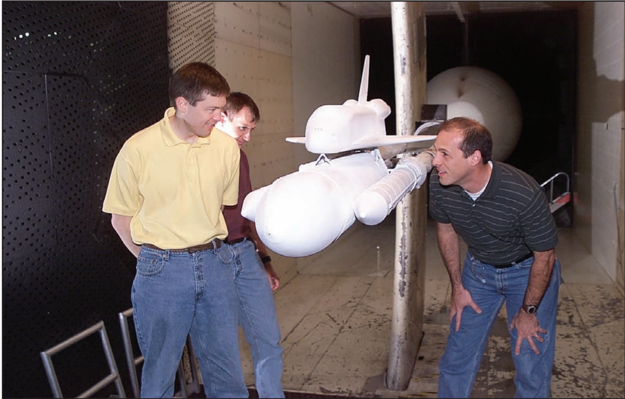
NASA personnel examine a shuttle model to be tested in AEDC's tunnel 16T.
