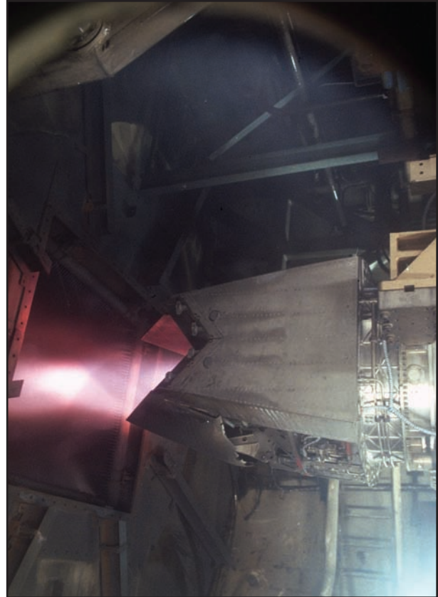
AEDC has conducted more than 9,000 hours of engine testing on the Pratt & Whitney F119 power plant for the F-22A Raptor.
