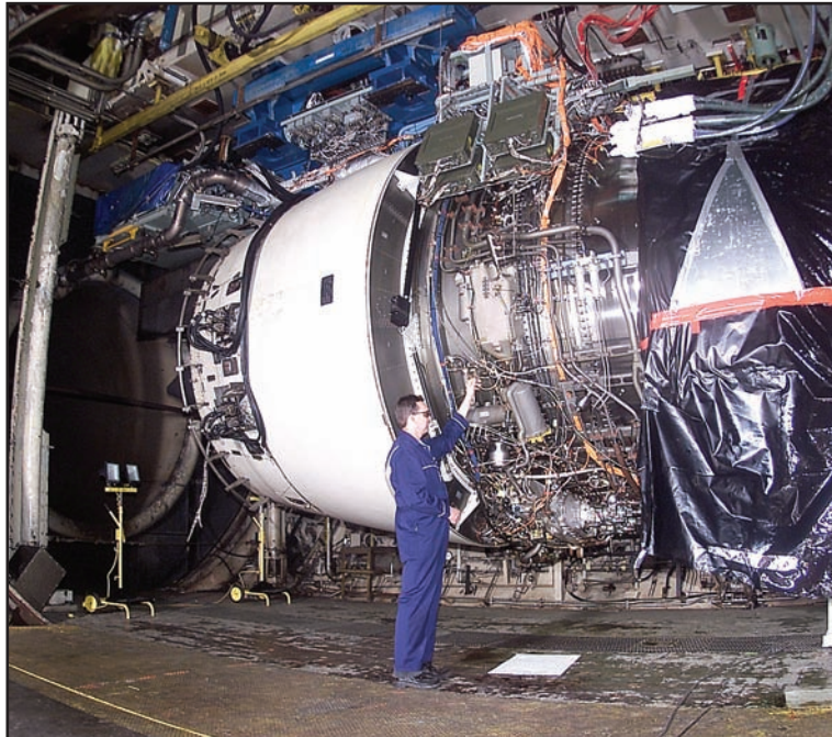
Left, a Rolls-Royce fitter checks instrumentation on the Trent 900 engine for testing in C-2. The engine, selected as a power plant for the Airbus A380 passenger aircraft, underwent engine operability, performance and icing tests. Above, Robert Saia, an executive vice president of the GE-P&W EA, speaks to assembled AEDC craftsmen and management personnel in ASTF test cell C-2 with the first EA GP7200 engine as his backdrop.
