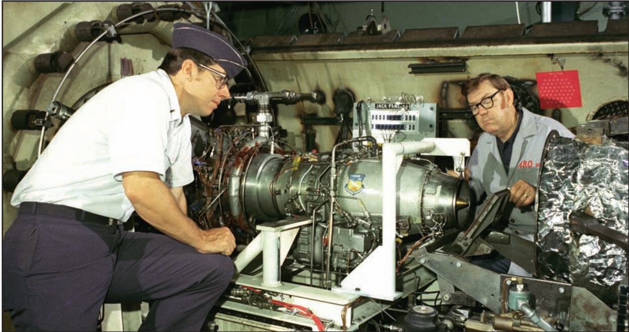
AEDC personnel check a quick-opening door at the F107 turbofan engine's exhaust nozzle. The door was opened as air was supplied to the engine's inlet to simulate an in-flight start.
