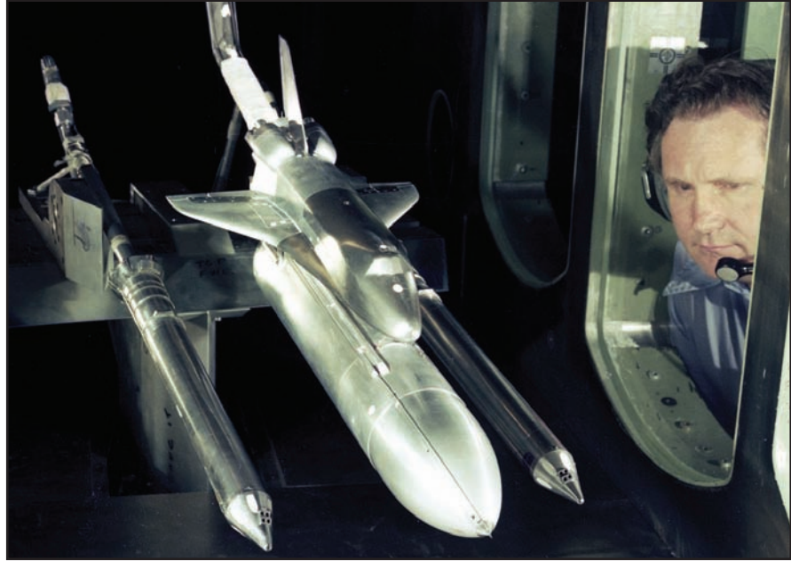
The scale model of the Space Transportation System (STS) is shown just before a staging test in hypersonic Tunnel A in the von Kármán Gas Dynamics Facility (VKF).
