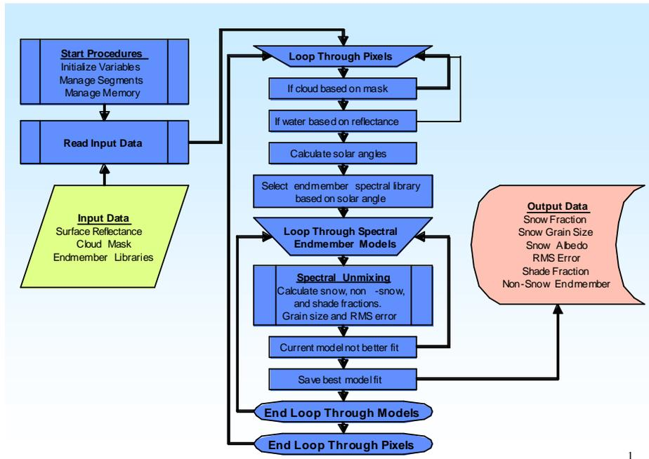
Figure 1. Basic flowchart of core snow cover elements in GOESRSCAG implementation.
