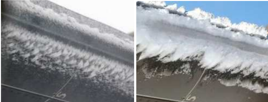
Figure 2: Ice accreted from super-cooled water droplets on the wing leading edge of a research aircraft while in cloud (Left) and after ascending above cloud (Right). Photo credits: NASA Glenn Research Center.
