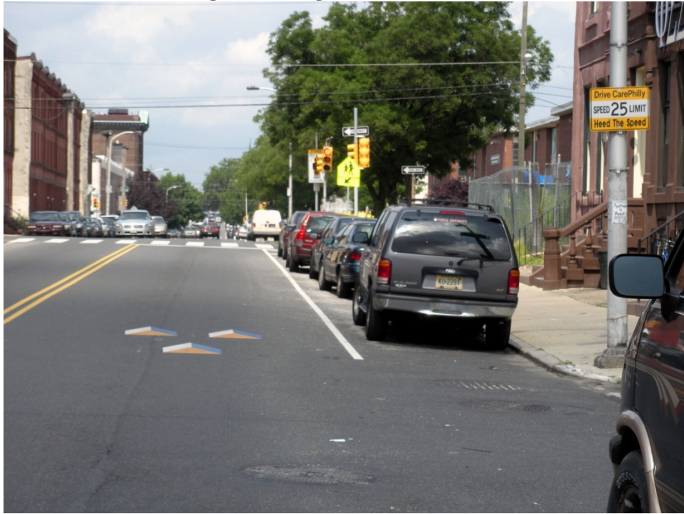
Figure 12. Sign and 3-D Installation
