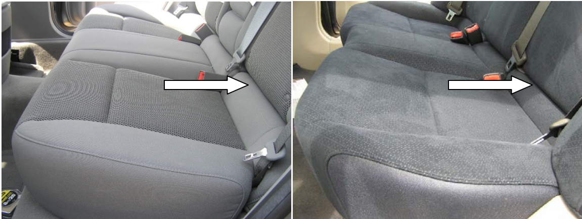
Figure 9. Illustration of vehicle seats with a bightline waterfall with vertical lower anchorage locations indicated.
