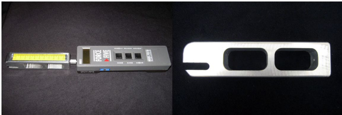
Figure 6. Tool to measure force required to engage lower anchorage (top view with force gauge on left and side view of connector portion on right).
