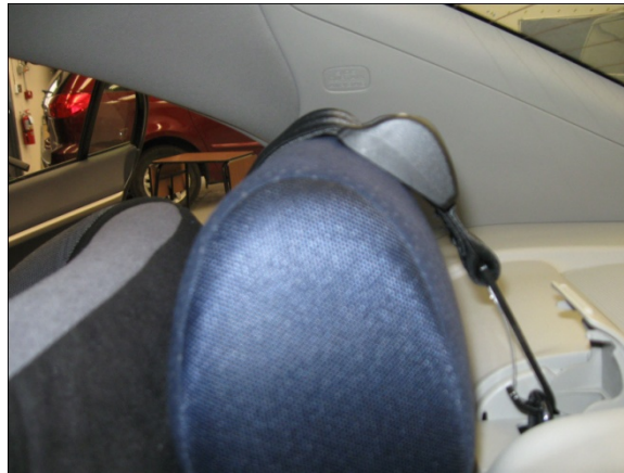
Figure 49. Incorrectly routed but tight tether installation.
