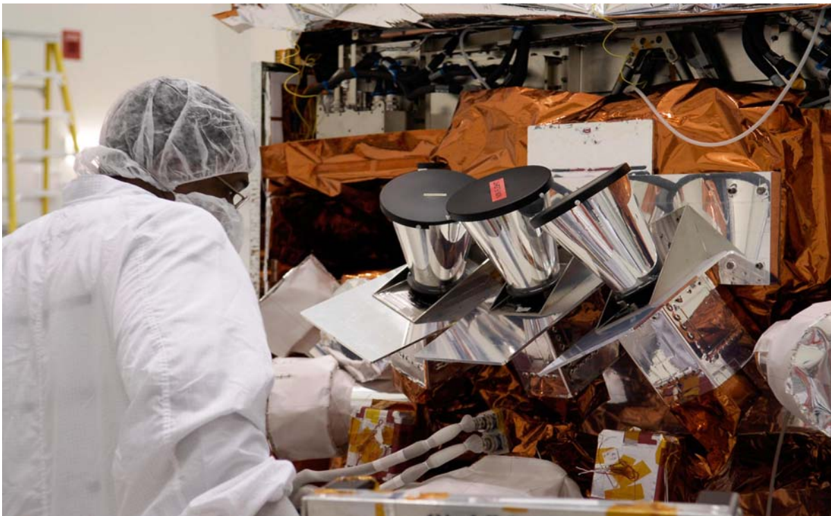
In April, Technicians checked the newly installed sun shades on GLAST's star trackers (near KSC) Credit: NASA/Kim Shiflett
