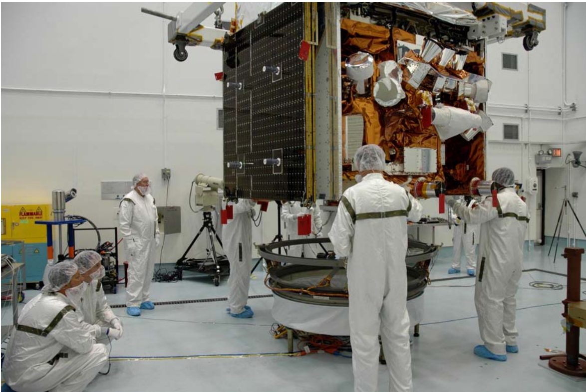
Technicians lower GLAST onto the payload attach fitting. Credit: NASA/Jim Grossmann
