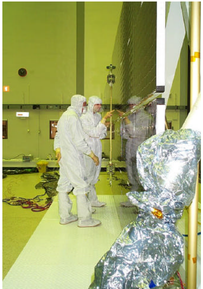
NASA engineers inspect cells on Hubble's new solar wing prior to testing. They find them in perfect condition.
