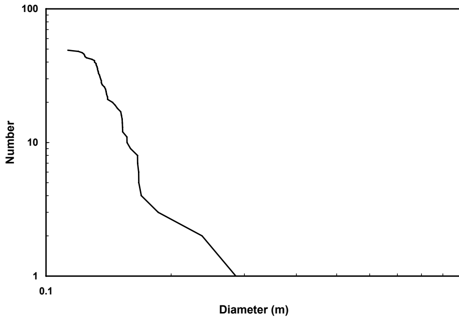
Figure 7.0-4. SEM size distribution for catalogued SNAPSHOT debris cloud candidate.
