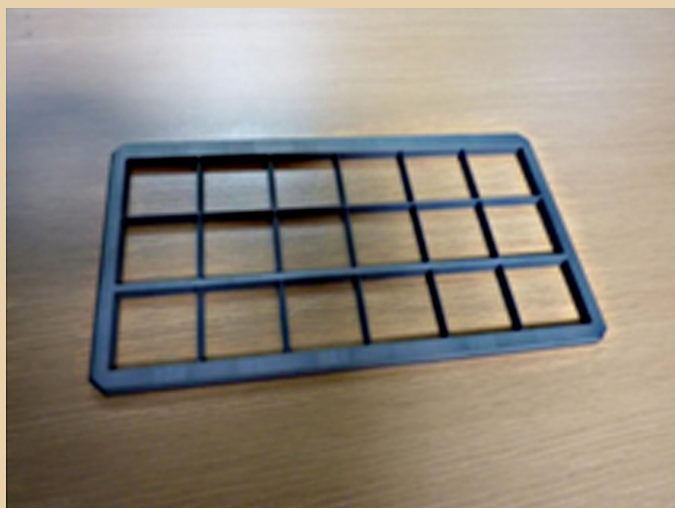
Figure 27. A photo of a prototype of the silicon carbide light shield for the EDU FPA is shown.
