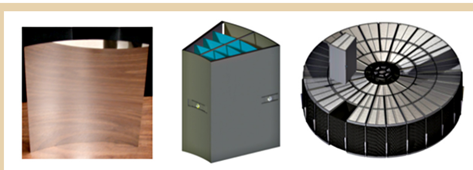
Figure 30. This graphic illustration shows the process of building an X-ray telescope. It starts with making many very thin mirror segments ( left ). Typically, on the order of 102 pairs of mirror segments are aligned and bonded into a mirror module ( middle ). Depending on the size of the telescope, tens to hundreds of modules are integrated to form a single telescope ( right ).
