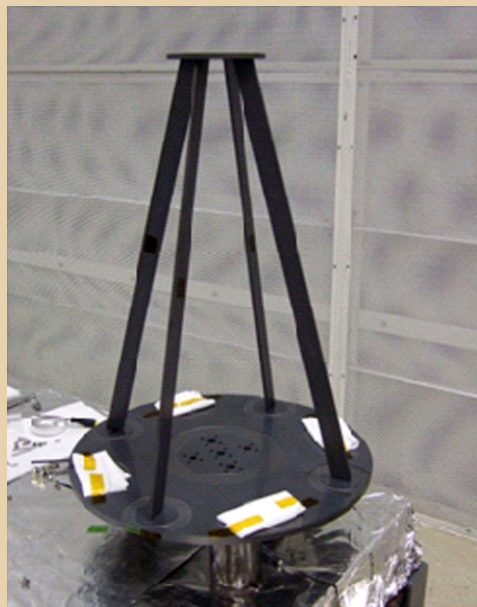
Figure 12. A silicon-carbide telescope spacer is shown with white paper to protect the polished mirror mounting pads.
