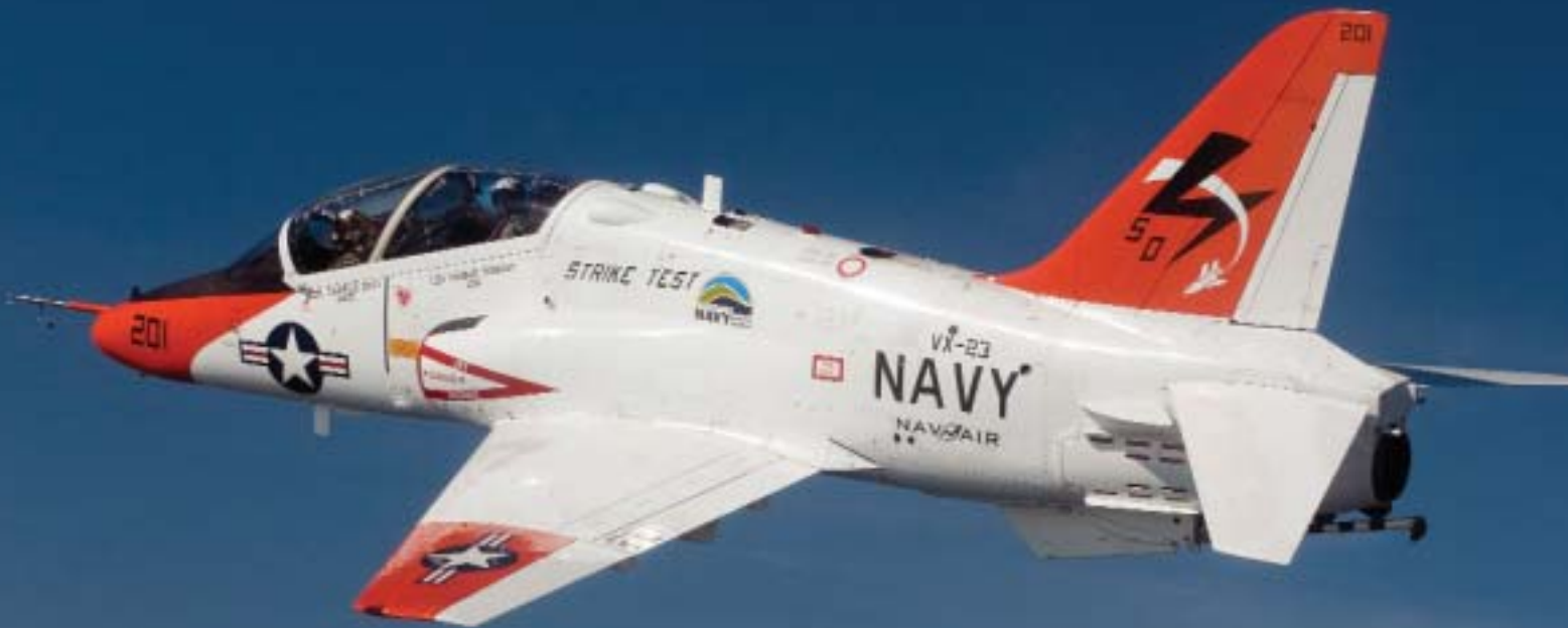
A T-45C Goshawk training aircraft conducts a test flight using a biofuel blend of JP-5 jet fuel and plant-based camelina.
