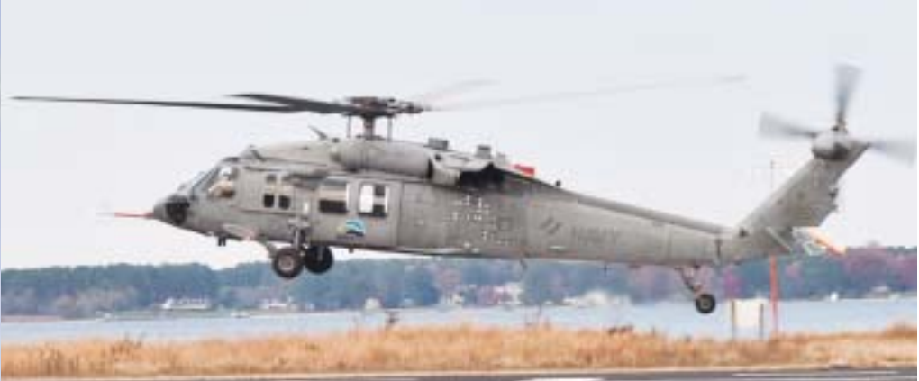
An MH-60S Seahawk helicopter tests a 50/50 Camelina seed-based biofuel blend at NAS Patuxent River. The test demonstrates another step toward the certification of fuels from non-petroleum sources for use in all Navy and Marine Corps aircraft. Sean Seremet
