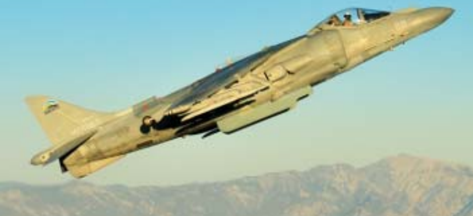
An AV-8B Harrier assigned to Air Test and Evaluation Squadron (VX) 31 conducts the first test flight of a mix of 50/50 jet fuel and biofuel. The test was conducted over Naval Air Warfare Center Weapons Division, China Lake.
