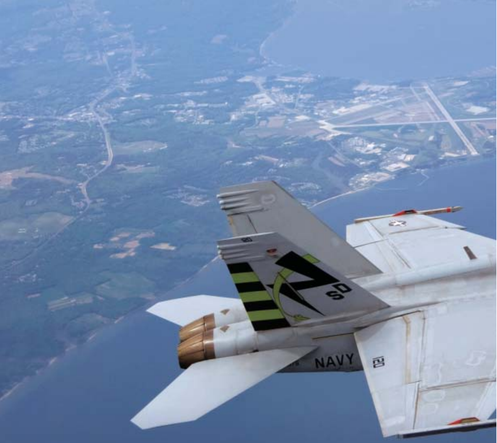
An F/A-18F Super Hornet strike fighter, dubbed the “Green Hornet,” conducts a supersonic test flight at Naval Air Station Patuxent River. The aircraft is fueled with a 50/50 Camelina seed-based biofuel blend. This Earth Day 2010 test drew hundreds of onlookers, including Secretary of the Navy Ray Mabus, who has made research, development, and increased use of alternative fuels a priority for the Navy.
