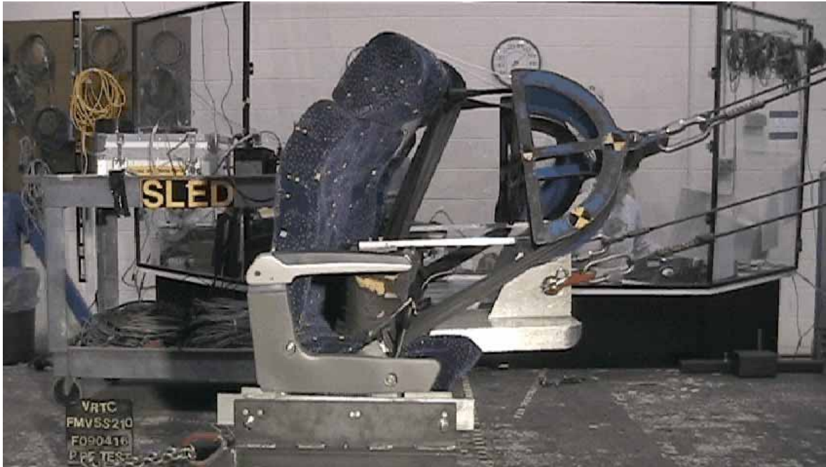
Figure 62 - Amaya 7G seat static test using floor and side rails
