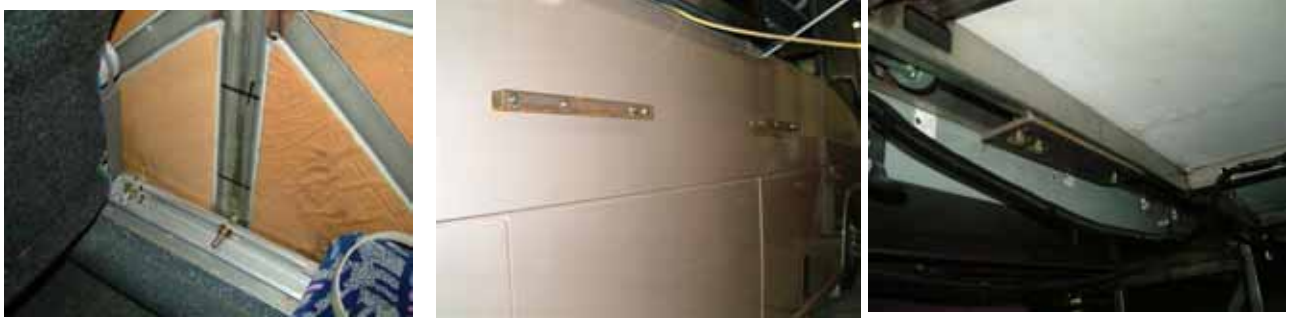
Figure 8 – Reinforced Seat Mountings for Rows 4R and 6R
