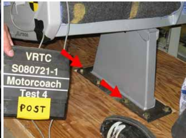
Figure 31 - Sled test setup with load cells at seat anchor of middle row seat
