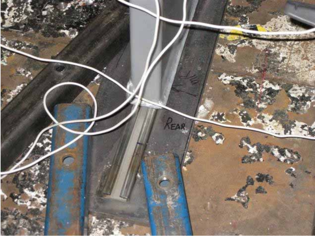
Figure 60 - Coach floor rail used in static test
