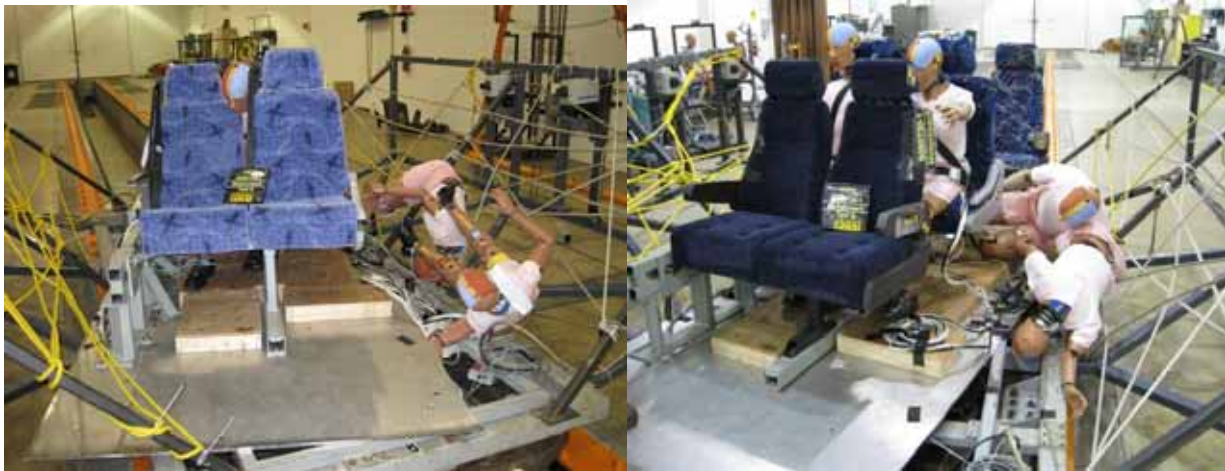
Figure 34 - Angled sled test post test dummy positions
