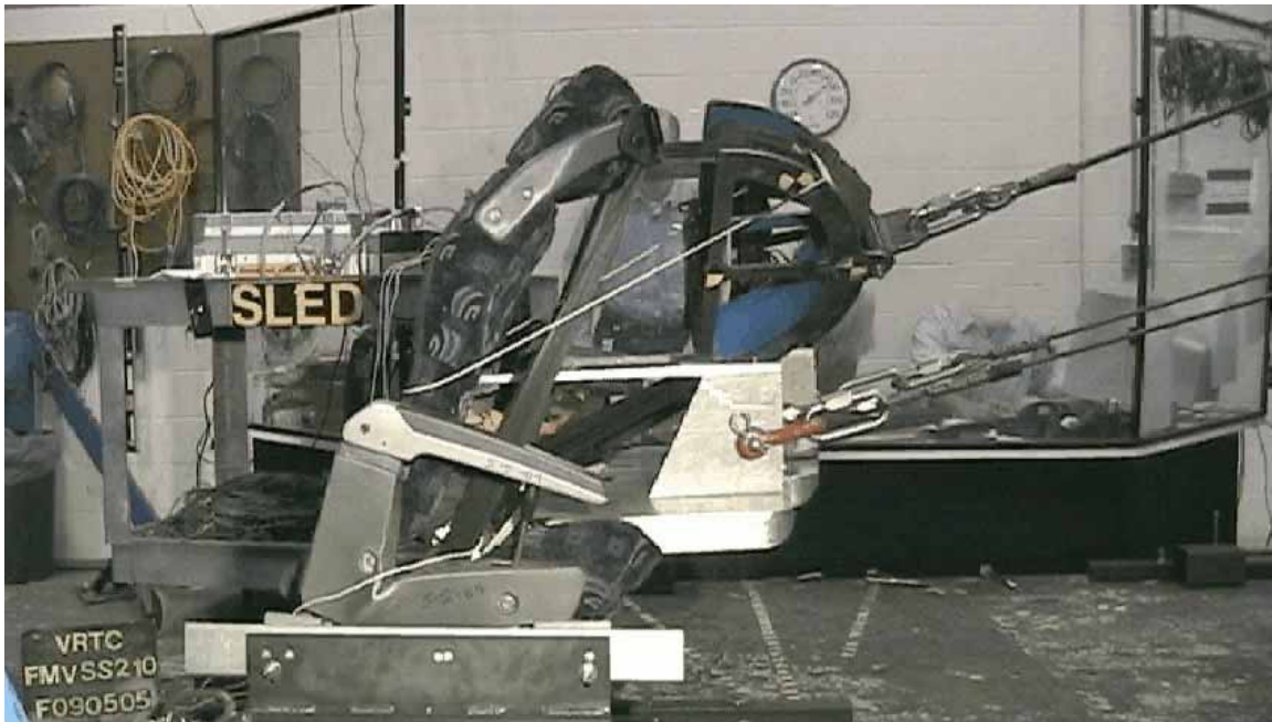
Figure 73 - Amaya 10G seat using new floor and side rails
