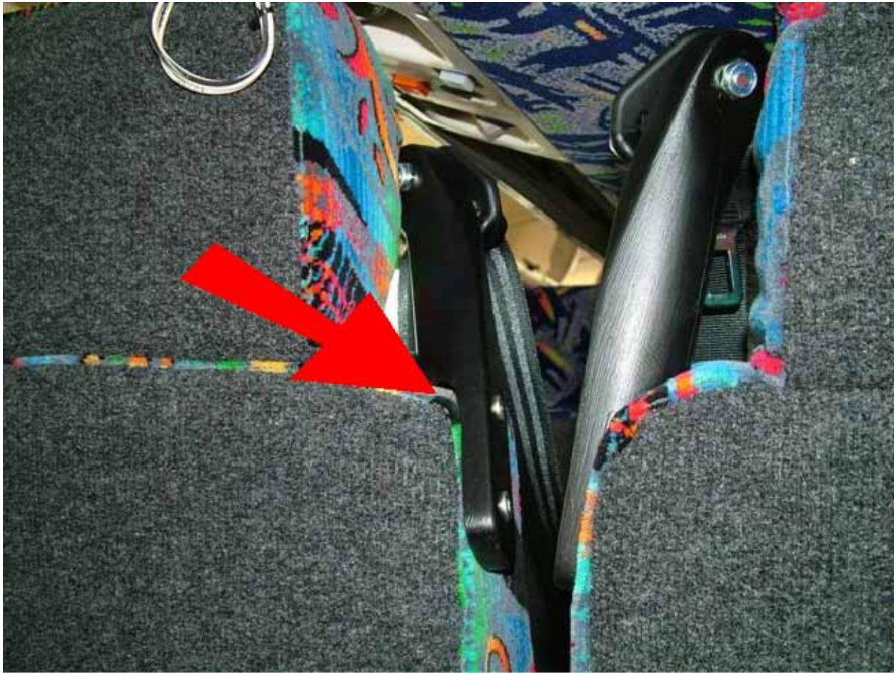
Figure 27 - Damage to D-ring mount
