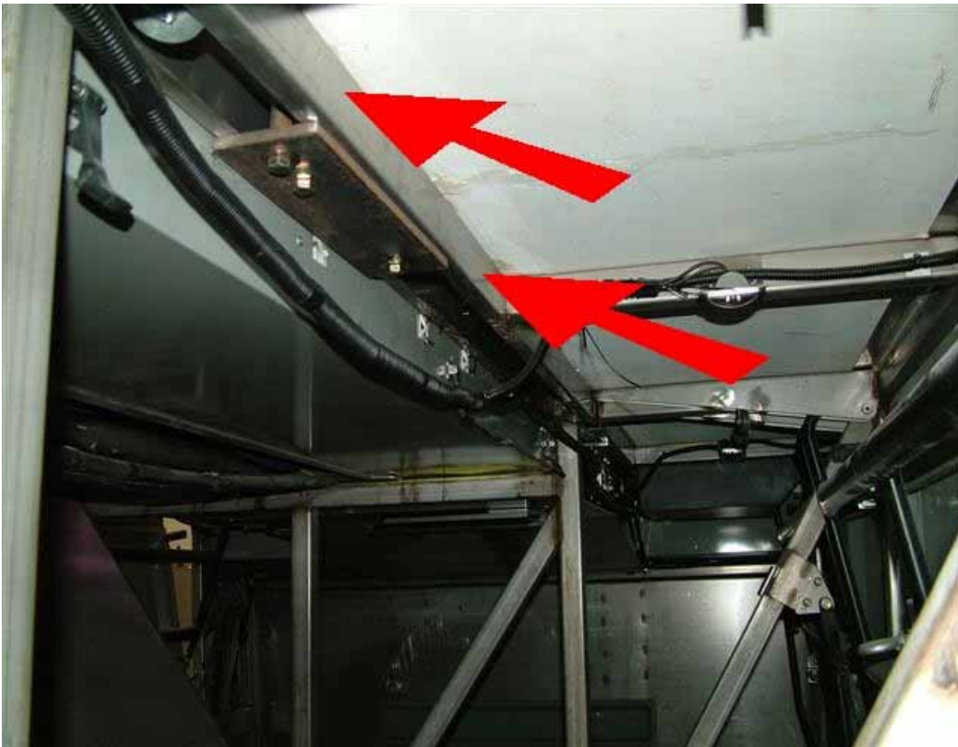
Figure 61 - Coach longitudinal floor-rail used to attach the seats
