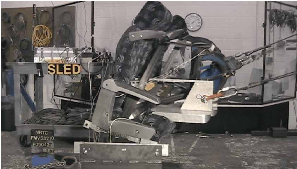
Figure 67 - Amaya 10G seat using floor and side rails used previously
