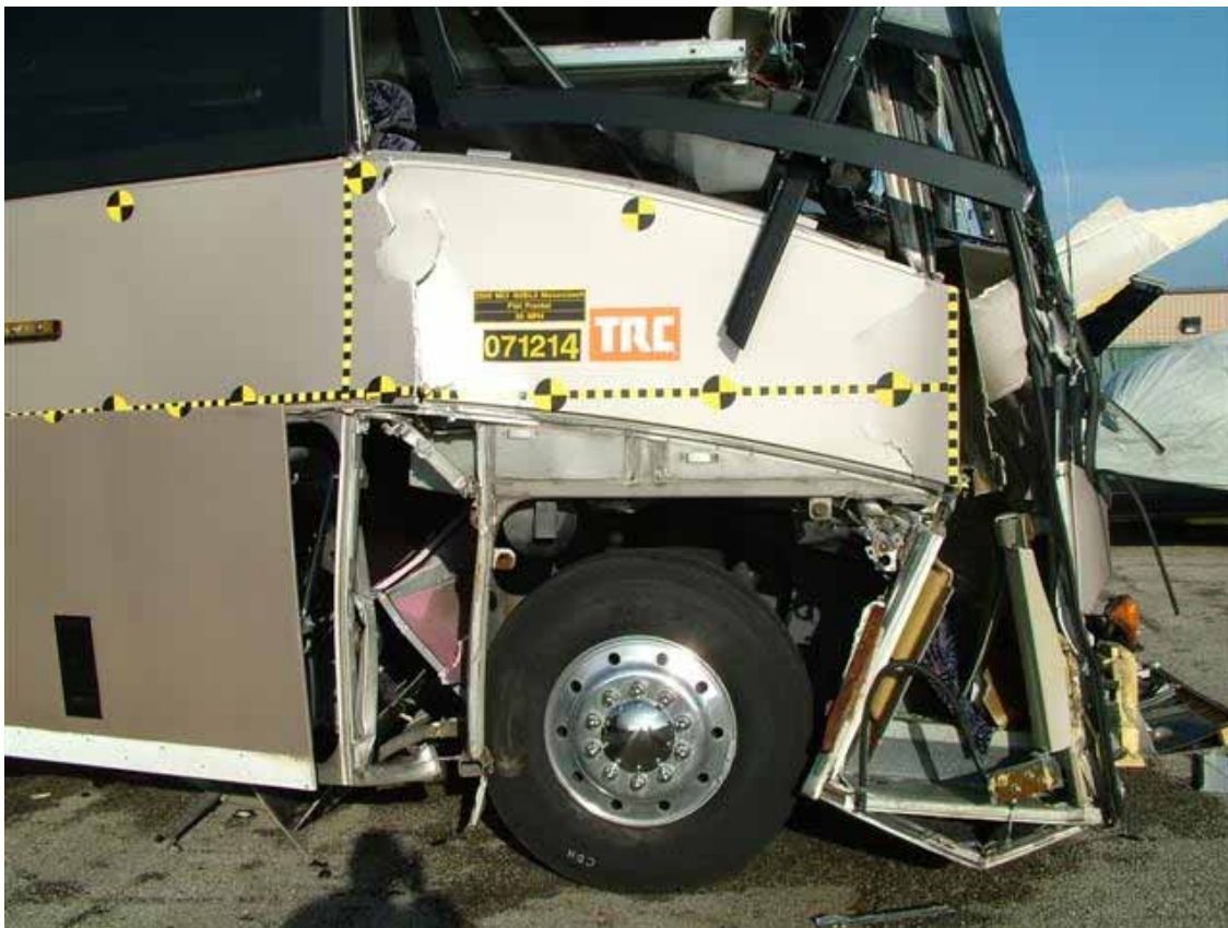
Figure 15 – Side View of Damage from Crash Test
