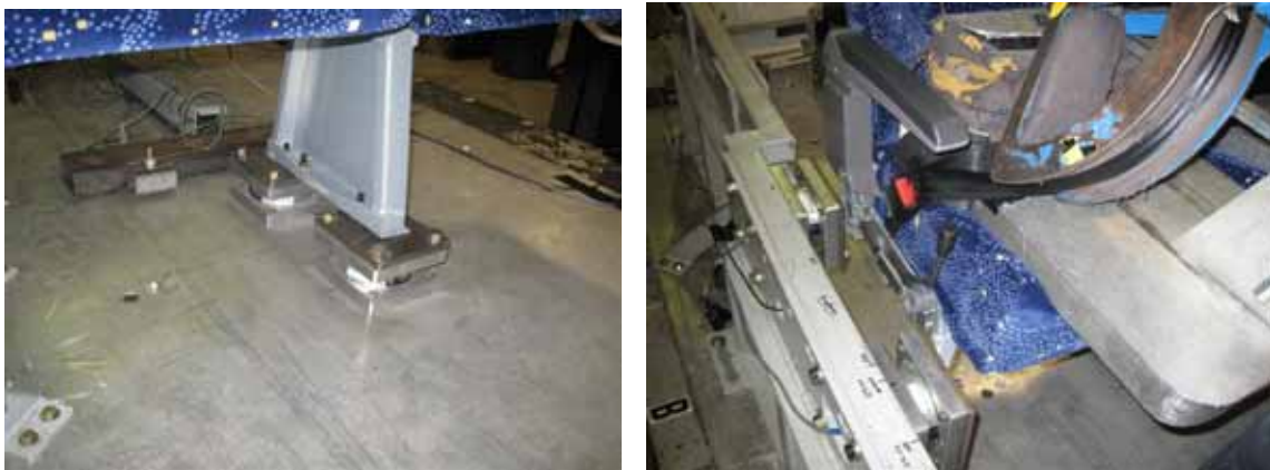
Figure 47 - Load cells at seat attachment points
