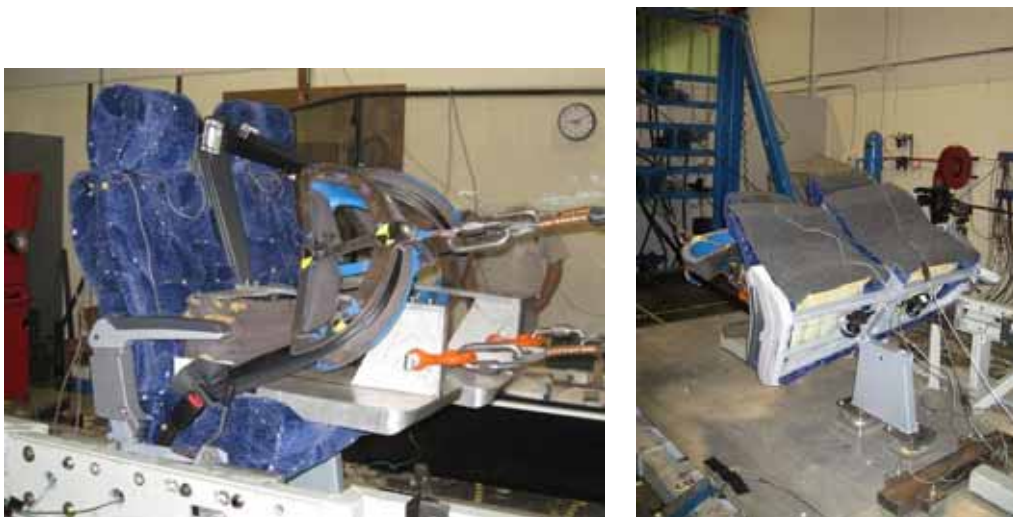
Figure 48 - Static pull and seat failure
