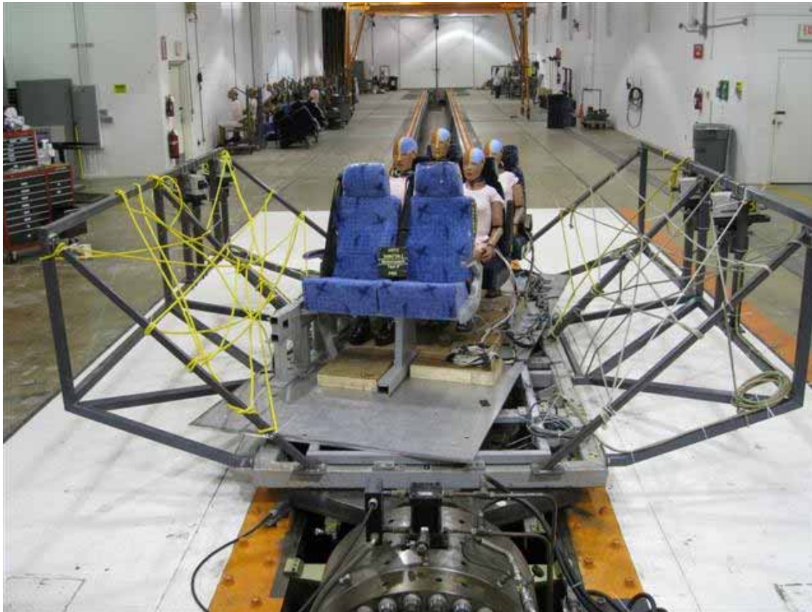
Figure 33 - Angled sled test setup
