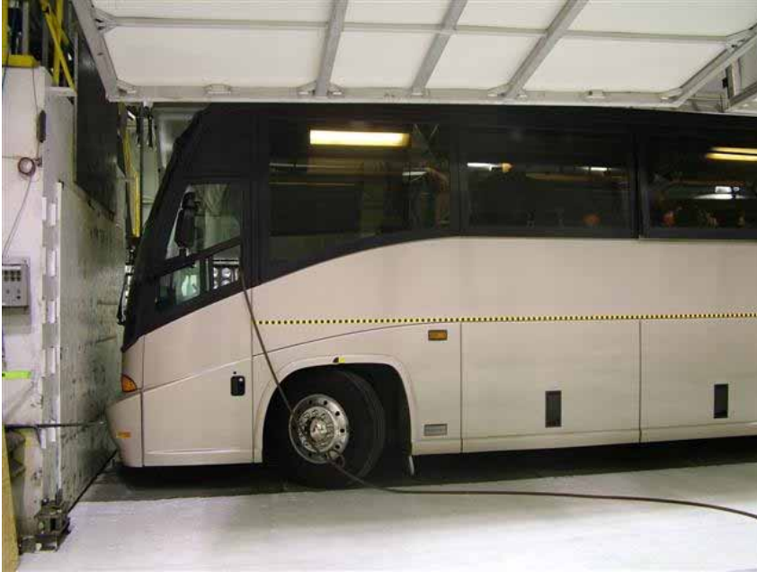
Figure 5 – Pre-Test Set-Up for Motorcoach Crash Test
