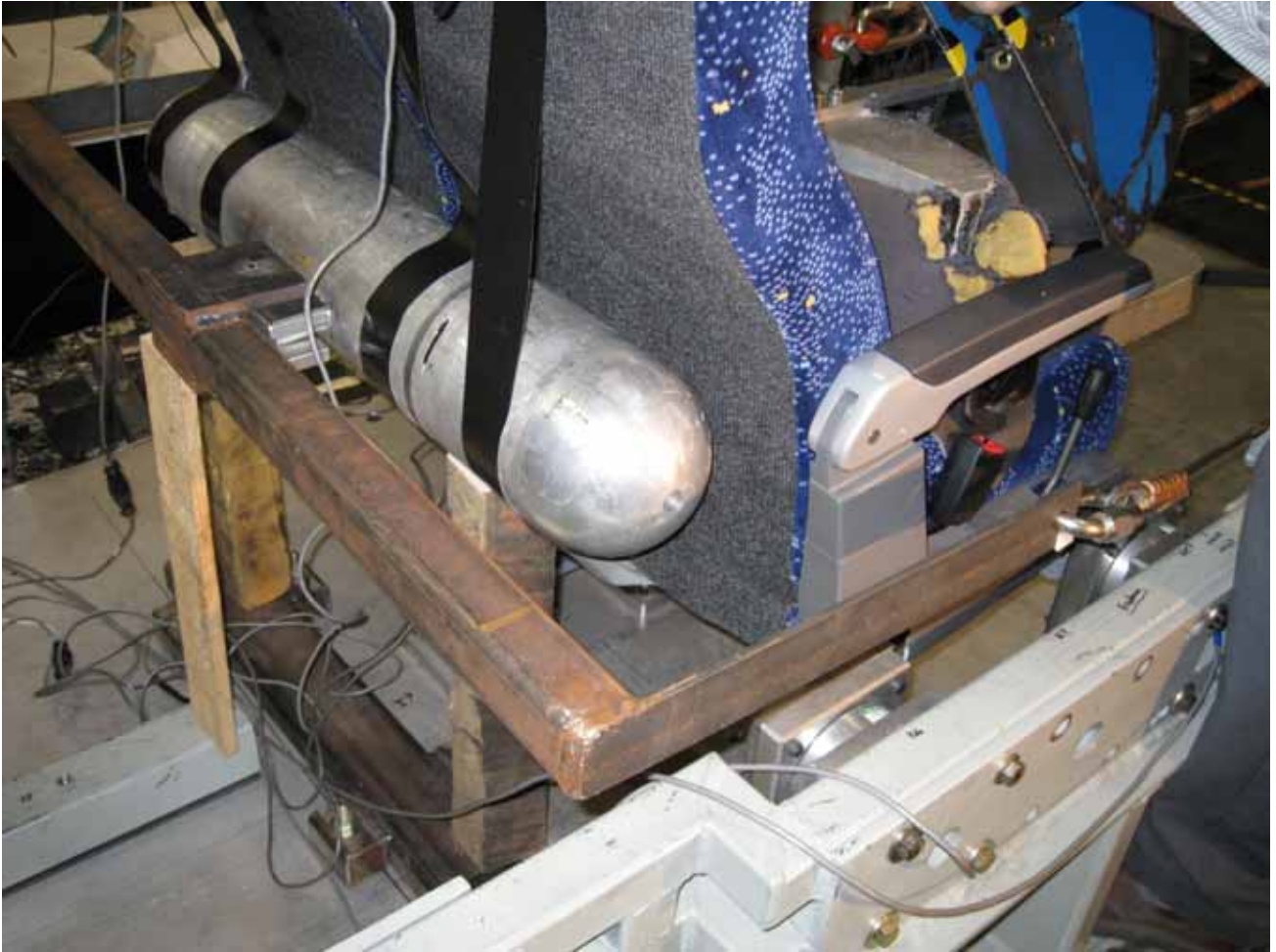
Figure 42 - Rear loading bar setup
