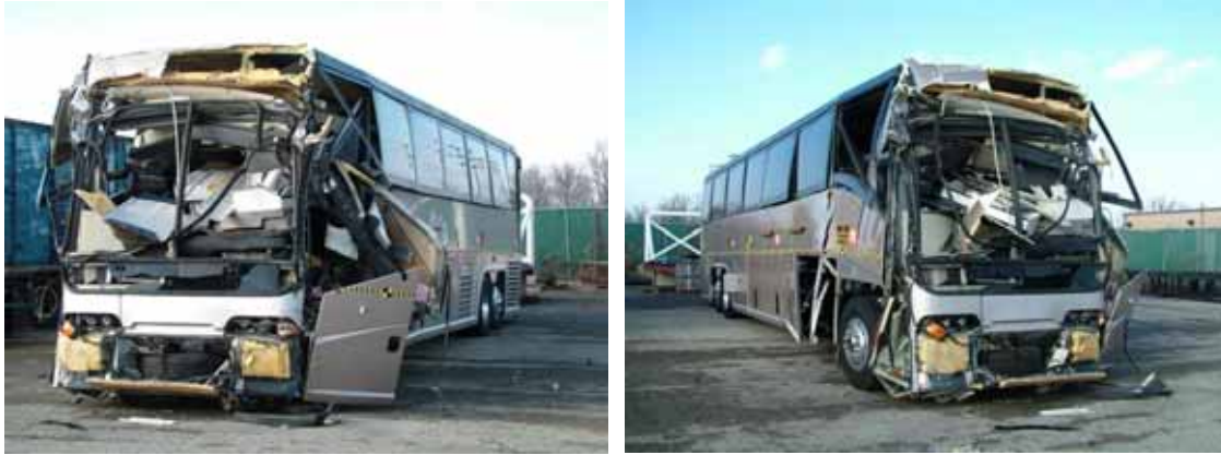
Figure 14 – Frontal Views of Damage from Crash Test
