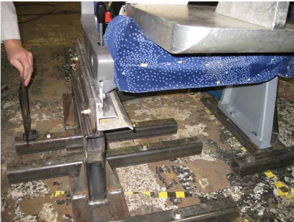
Figure 59 - Coach side rail used in static test
