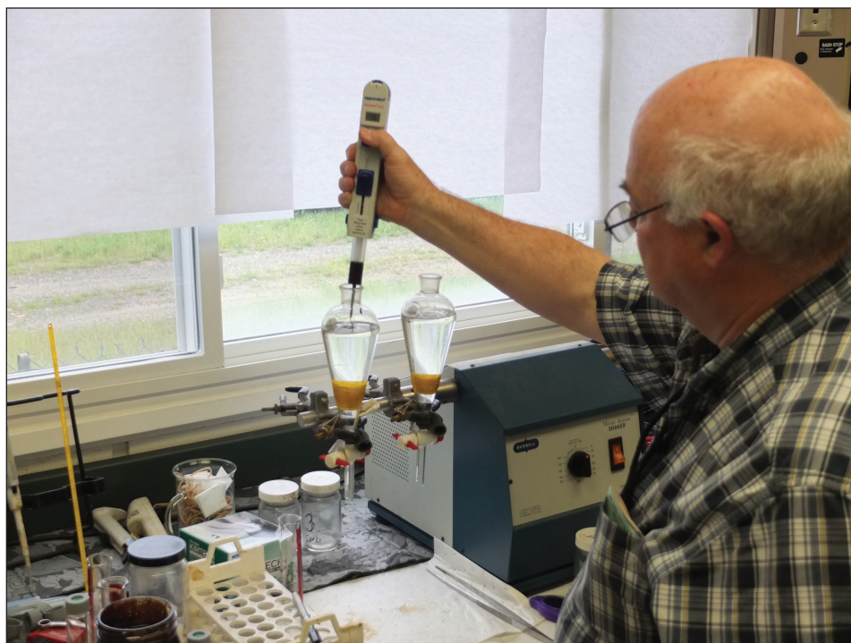
Ken Trudel of S.L. Ross Environmental Research, Ltd. tests the dispersed oil/water samples in the Ohmsett laboratory.
