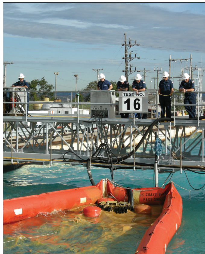
U.S. Coast Guard National Strike Force Team members train with the new Desmi Helix brush skimmers. Each NSF team will receive the new skimmers in the upcoming year.
