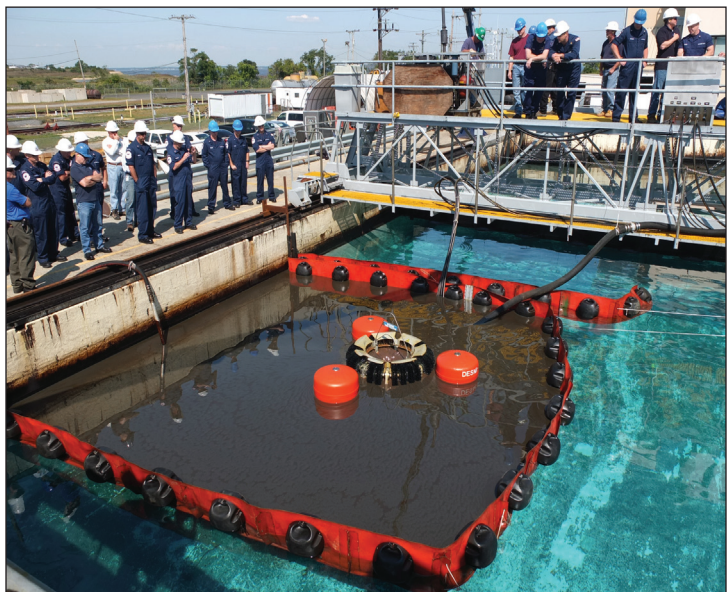
The DOP Dual Helix Brush skimmer was tested for overall performance using the ASTM F2709 Standard Test Method for Determining Nameplate Recovery Rate of Stationary Oil Skimmer Systems. The U.S. Coast Guard recently acquired the latest generation of the Desmi skimmer.
