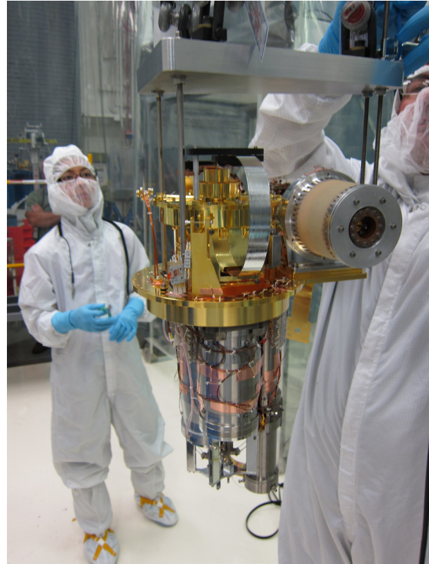
The engineering model of the detector and cooling stage for the Astro-H Soft X-Ray Spectrometer. The cooling stage consists of a three-stage adiabatic demagnetization refrigerator that cools the 36-pixel array to 50 mK for more than 40 hours at a time before needing to be recycled for about 1 hour. The detector system achieved an energy resolution of about 4.5 eV.
