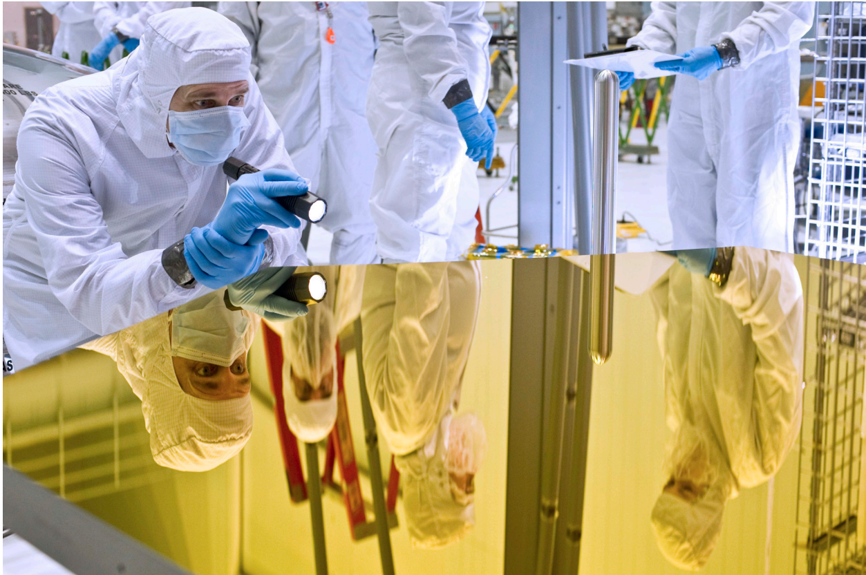
The gold-coated primary mirror segment engineering design unit (EDU) is inspected at Goddard Space Flight Center, Md. NASA/Chris Gunn
