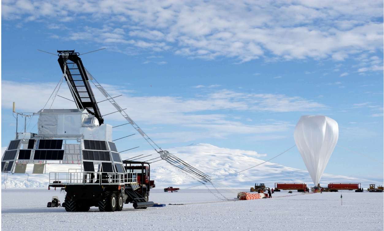
BESS-Polar II prepares for launch from Williams Field near McMurdo Station, Antarctica, in Dec. 2007. BESS-Polar II flew for 24.5 days with the superconducting magnet energized and measured over 4.7 billion cosmic ray events.
