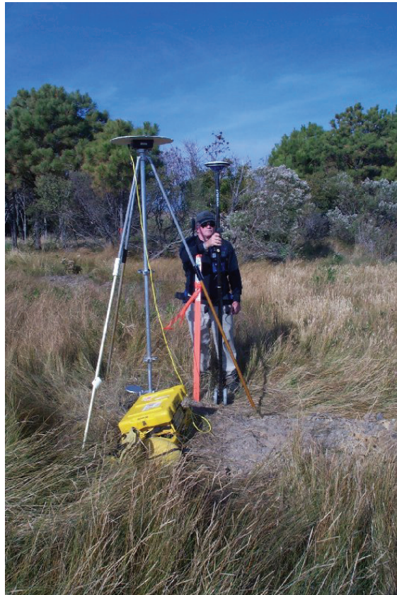
Diagram II-1. The base station should use a ground plane, choke ring, or a current high quality, geodetic, multipath rejecting antenna while the rover typically operates with a smaller antenna (usually integrated with the rover receiver) for ease of use.
