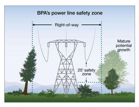
BPA crews will maintain a 25-foot safety zone between the highest point the vegetation will potentially grow and the lowest point the power line will sag under extreme conditions. Sometimes, even though a tree is outside the right-of-way boundary, BPA crews will remove any growth that comes within the 25-foot clearance zone or remove the tree if it's unstable and likely to topple over on the power line.
