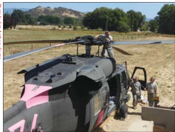
Soldiers from Forward Support Company, 579th Engineer Battalion, work Sept. 12 to remove the rotor blades from a UH-60 Black Hawk that had experienced a transmission problem while fighting fires near this clearing in Lakeport, Calif.
