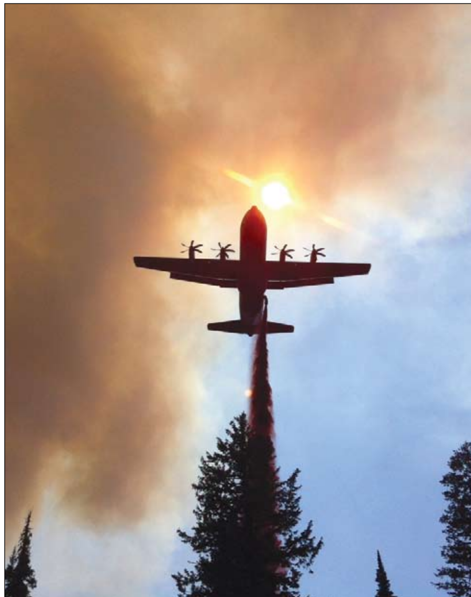
The California National Guard fulfilled a wide variety of missions around the globe and around the country in 2012, including dropping millions of gallons of water and fire retardant on wildfires in California and other U.S. locations. Above, a Modular Airborne Firefighting Systems II-equipped C-130J airplane from the Cal Guard's 146th Airlift Wing drops retardant on a fire near Twin Falls, Idaho, on Aug. 8. Photo by Mike Freer
