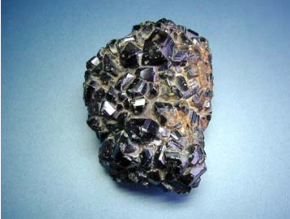
Sample of cassiterite, primary ore mineral for tin. Image from Minerals in Your World .
