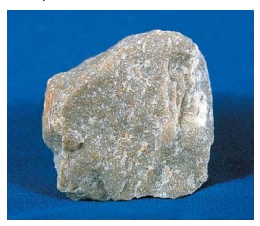
Silica (SiO2) as quartz or quartzite (shown here) is used to produce silicon ferroalloys for the iron and steel industries, and silicon metal for the aluminum and chemical industries. Image from *Minerals in Your World*.
