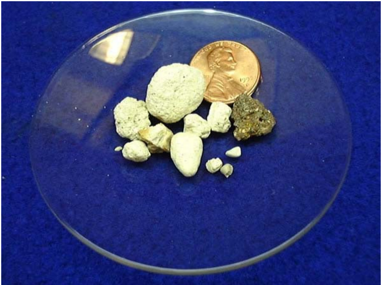
Samples of phosphate rock with penny for scale. Image from Minerals in Your World .
