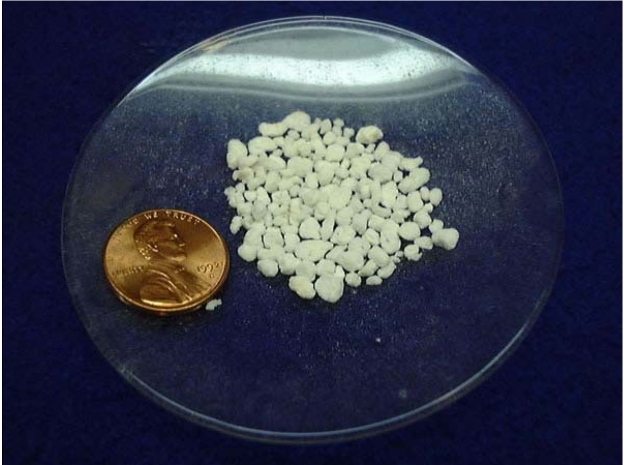
Sample of expanded perlite with penny for scale. Image from Minerals in Your World .
