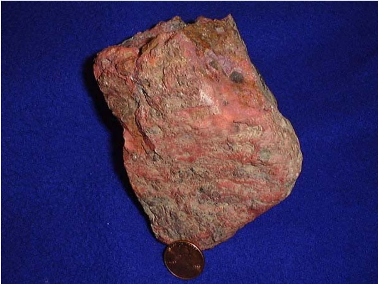
Sample of cinnabar, primary ore of mercury. Image from Minerals in Your World .
