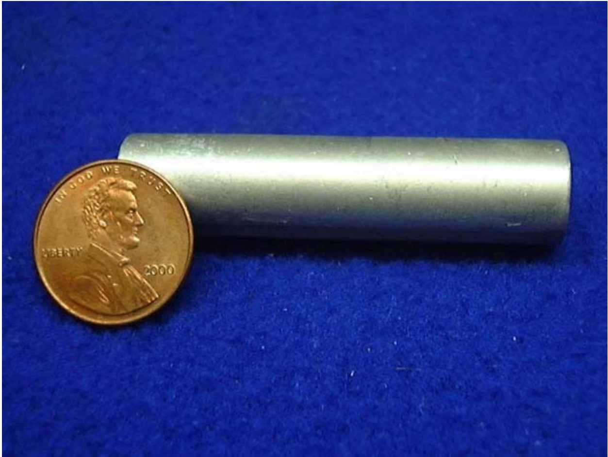
Sample of magnesium metal with penny for scale. Image from Minerals in Your World .
