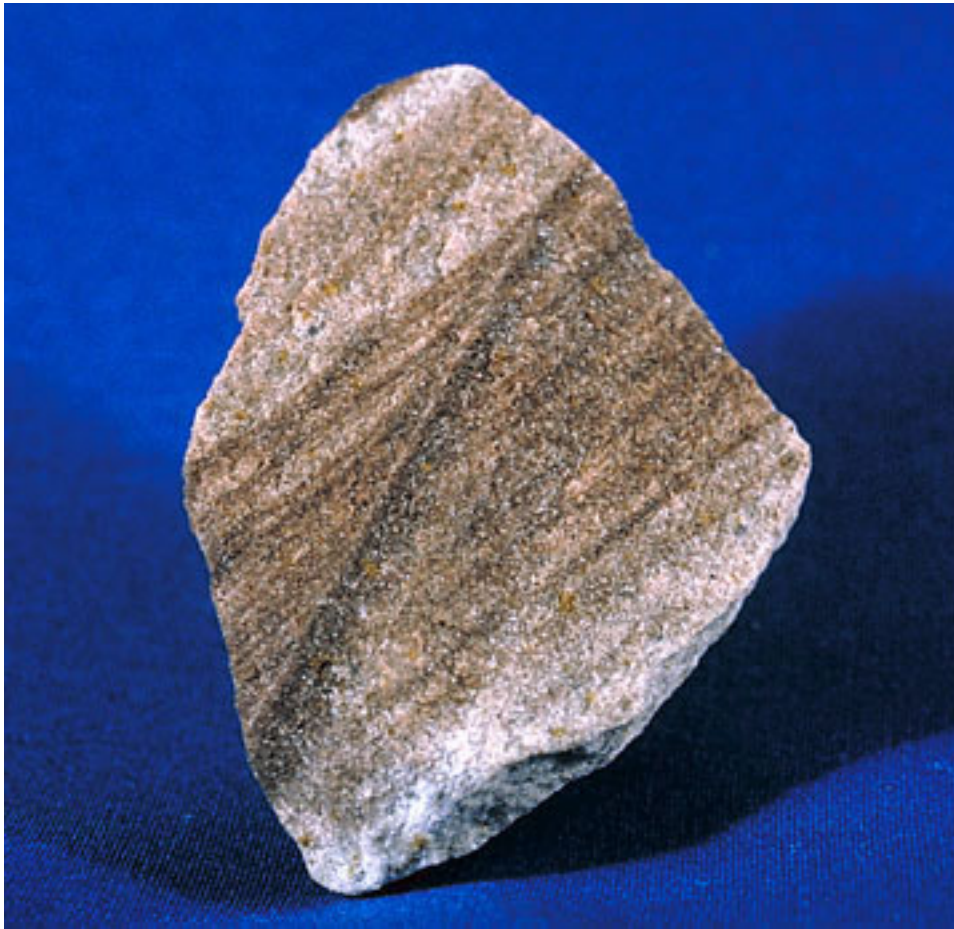
Quartz sandstone, a source of industrial sand and gravel. Image from Minerals in Your World .
