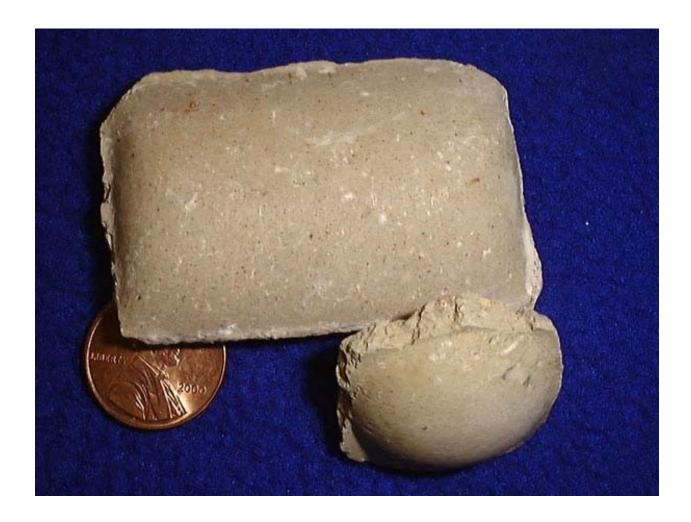
Sample of fluorspar, a common commercial term used to describe concentrates of fluorite (penny for scale). Image from *Minerals in Your World*.
