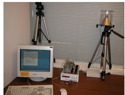
Figure 2. Testbed transmitter, antenna, and GPS.
