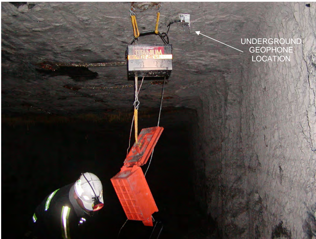
Figure 10. Underground Geophone Location.
