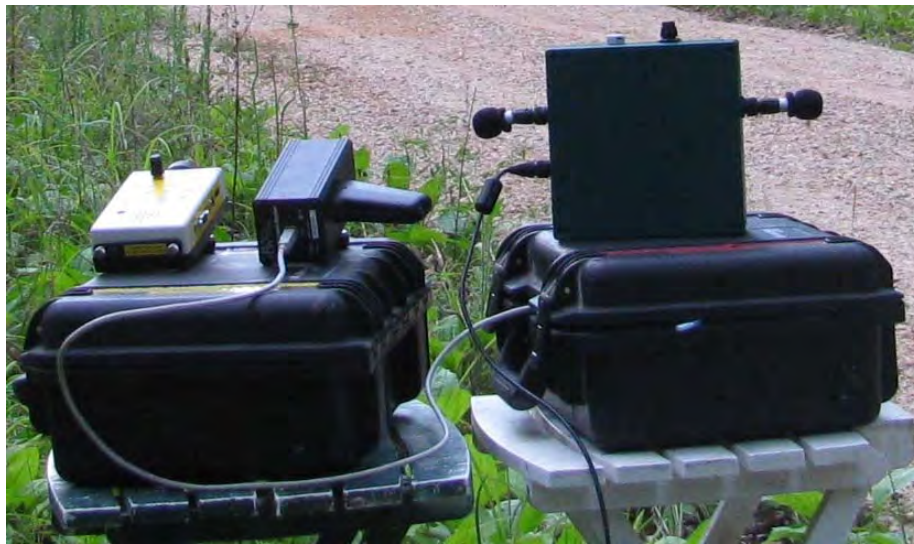
Figure 1. Setup of detector comparison. Anabat SD1 on left in this example, AR125 with FR125 in the middle, and SM2BAT on the right.
