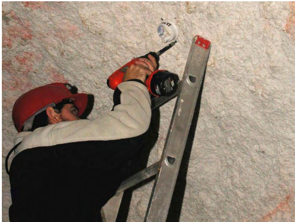
Figure 5. Installation of data logger.
