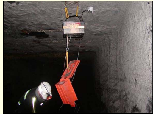
Deep Mine Geophone Installation
