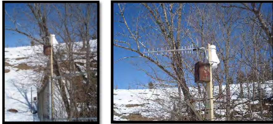
Figure 16: Acoustical Data Capture System at Hellhole Cave
