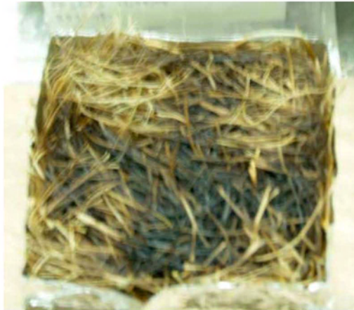
Figure 44. This slightly out of focus photograph shows the top surface of a May tall fescue fuel bed following application of an applied radiative heat flux that was insufficient to induce glowing combustion.
