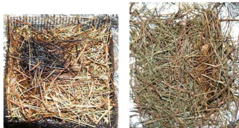
Figure 68. Bottom (left) and top (right) views of a May tall fescue/pine needle mixed fuel bed are shown after the fuel was removed from the heated plate held at 320 °C with a high wind applied. No glowing combustion was observed.
