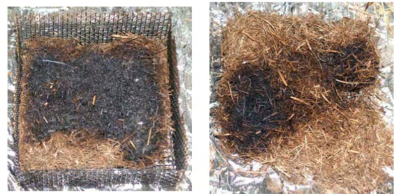
Figure 57. Bottom (left) and top (right) views of a fine Florida grass fuel bed are shown after the fuel was removed from the heated plate held at 321 °C with no wind applied. Glowing combustion was observed.
