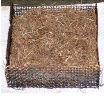
Figure 17. Photograph of fine Florida grass in wire-screen cage.
