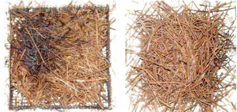
Figure 62. Bottom (left) and top (right) views of a pine needle fuel bed are shown after the fuel was removed from the heated plate held at 340 °C with no wind applied. No glowing combustion was observed.
