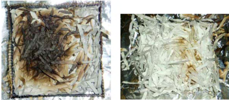
Figure 25. Bottom (left) and top (right) views of a shredded newsprint fuel bed are shown after the fuel was removed from the heated plate held at 333 °C with a low wind applied. Glowing combustion was not observed.
