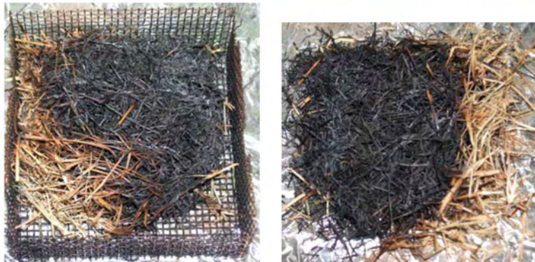
Figure 49. Bottom (left) and top (right) views of an August tall fescue fuel bed are shown after the fuel was removed from the heated plate held at 310 °C with a low wind applied. Glowing combustion and flaming were observed.
