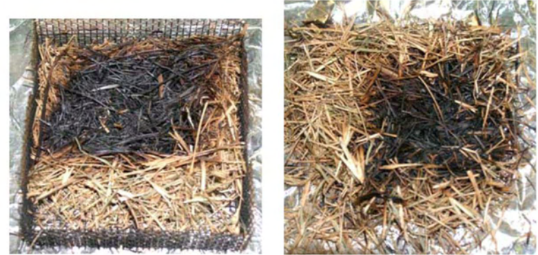
Figure 47. Bottom (left) and top (right) views of an August tall fescue fuel bed are shown after the fuel was removed from the heated plate held at 300 °C with no wind applied. No glowing combustion was observed.
