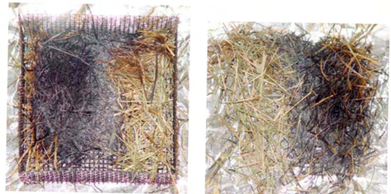
Figure 35. Bottom (left) and top (right) views of a May tall fescue fuel bed are shown after the fuel was removed from the heated plate held at 336 °C with a high wind applied. Glowing combustion was observed after 134 s.
