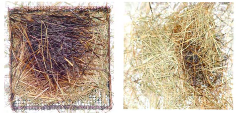
Figure 37. Bottom (left) and top (right) views of a May tall fescue fuel bed are shown after the fuel was removed from the heated plate held at 311 °C with a low wind applied. Glowing combustion was not observed.
