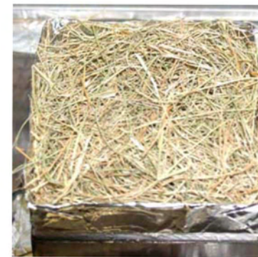
Figure 11. A sample holder used during the radiative ignition experiments is shown filled with fuel.
