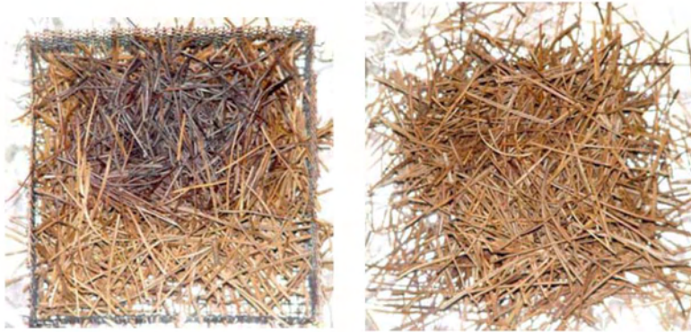
Figure 61. Bottom (left) and top (right) views of a pine needle fuel bed are shown after the fuel was removed from the heated plate held at 290 °C with no wind applied. No glowing combustion was observed.
