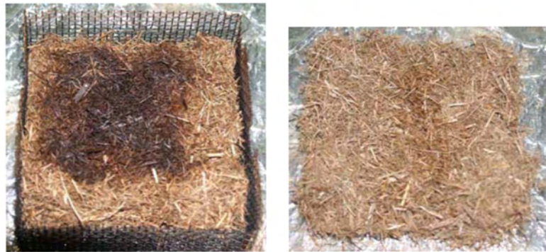
Figure 59. Bottom (left) and top (right) views of a fine Florida grass fuel bed are shown after the fuel was removed from the heated plate held at 290 °C with a low wind applied. Glowing combustion was not observed.
