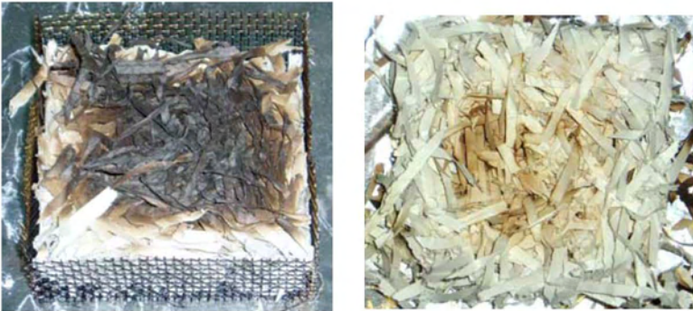
Figure 26. Bottom (left) and top (right) views of a shredded newsprint fuel bed are shown after the fuel was removed from the heated plate held at 332 °C with no wind applied. Glowing combustion was not observed.
