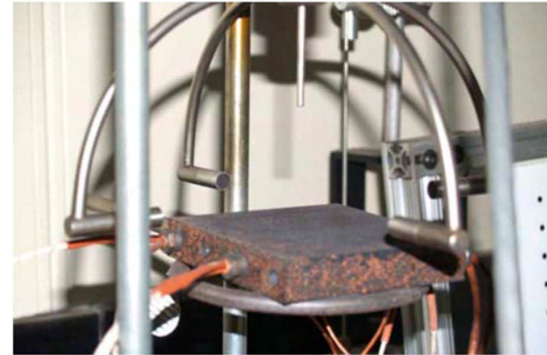
Figure 4. Photograph showing the sonic anemometer probe used to characterize the applied wind velocity in place 1.2 cm above the unheated copper plate.
