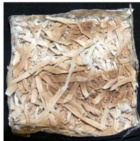
Figure 32. Photograph of the top surface of a shredded newspaper fuel bed following application of a 7.5 kW/m 2 heat flux.
