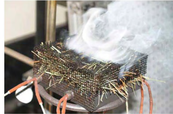
Figure 23. The smoke generated by a mixture of May tall fescue and pine needles applied to the heated plate at 380 °C in the presence of a low wind is shown 175 s after application.
