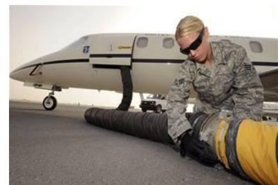
Connecting AC hoses to a C-21
