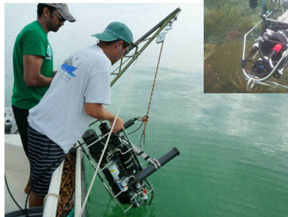
Launching optical profiler where it will collect gas emission data from the ocean floor.
