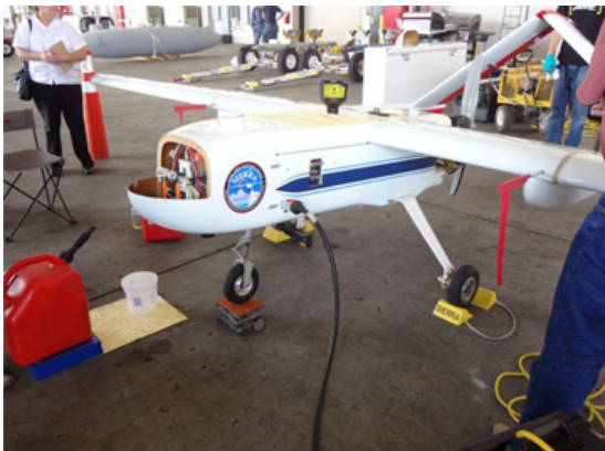
Nose of aircraft removed to inspect payload.
