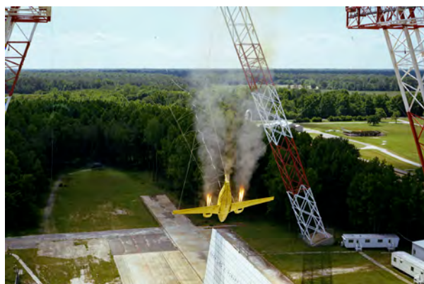
Full-scale impact testing in 1979.
