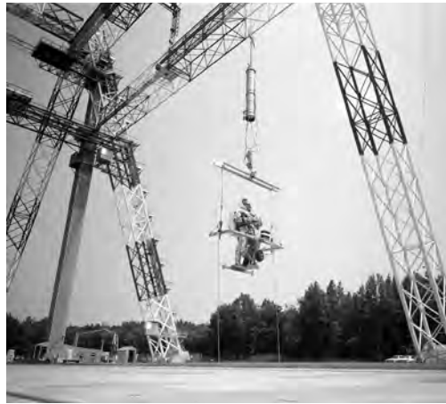
A 1967 POGO flying vehicle test.
