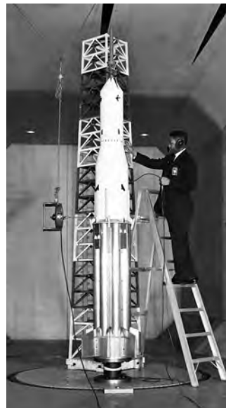
Engineer Tom Brydsong checks the Apollo/Saturn 1B Ground-wind-loads model in the NASA Langley Transonic Dynamics Tunnel.
