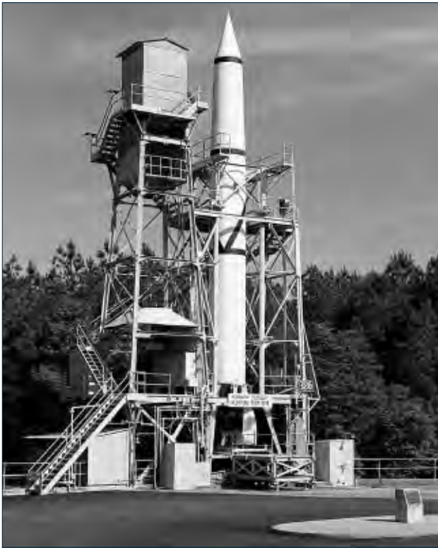
The Redstone Test Stand, used in the 1950s in the early development of the Redstone missile propulsion system, static tested the Redstone missile that launched Alan Shepard into space.
