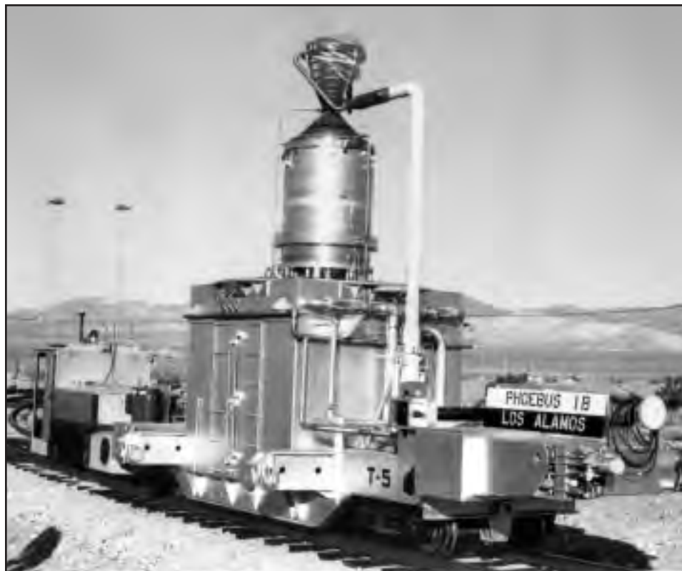
The Phobos 1B nuclear thermal rocket engine test reactor was created to further redefine the engineering aspects of a nuclear propulsion system. This particular unit was successfully tested in 1967.
