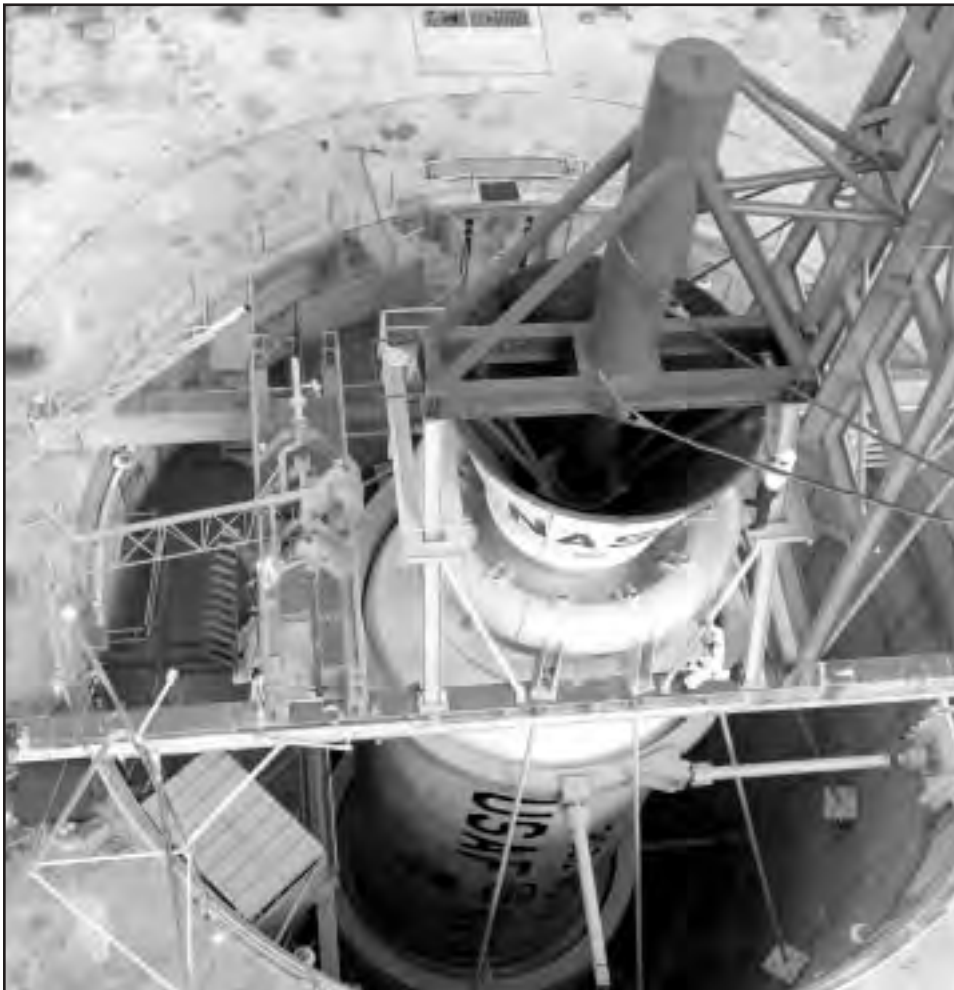
The SL-2, one of NASA's large solid rocket motors, generated over 3.6 million pounds of thrust on 23 February 1966. The 22-foot-diameter, 80-foot-long rocket contained 1.7 million pounds of solid propellant.
