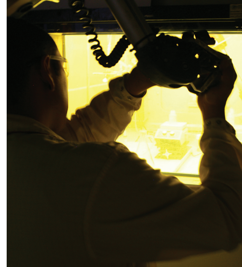
Matt Quintana uses remote manipulator arms to handle target discs that contain newly formed radioactive isotopes.
