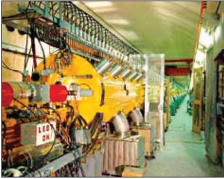
Brookhaven's 200-megaelectronvolt linear accelerator provides protons for use at the Brookhaven Linac Isotope Producer.
