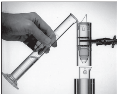
Brookhaven National Laboratory's first (circa 1950s) experimental technetium-99m generator with molybdenum-99 sorbed on alumina.
